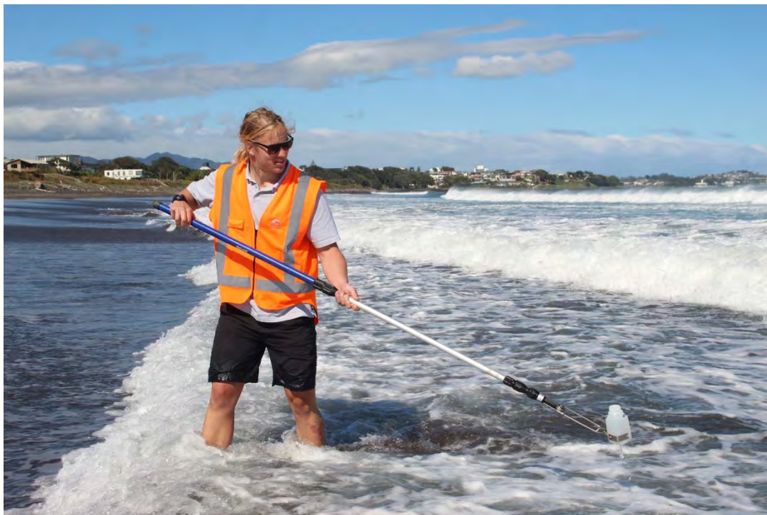
Photo 6 A bacteriological water quality sample being collected at the Fitzroy site (August 2016)
