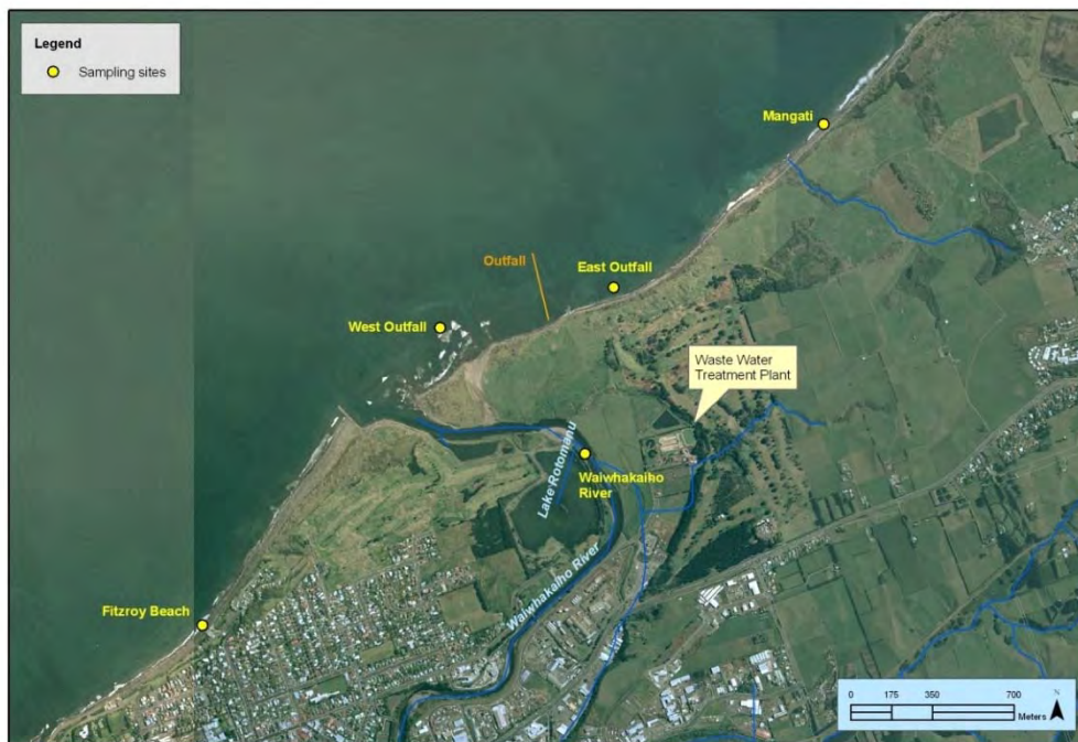
Figure 18 Locations of monitoring sites in relation to the NPWWTP
