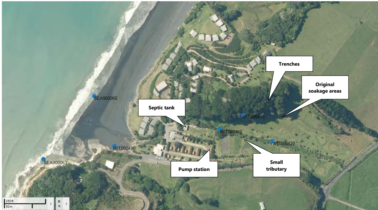
Figure 1 Location of sewage treatment system and sampling sites at the Wai-iti Beach Retreat
