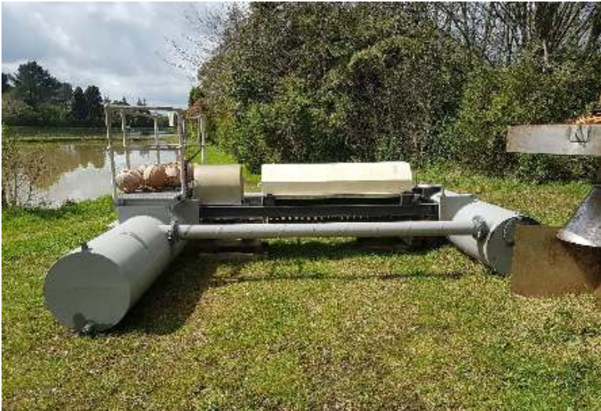
Photo 2 Aeration boom removed for maintenance, July 2017
