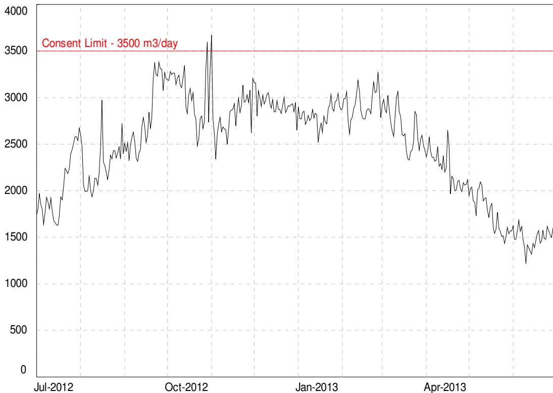
Figure 16 Graph of the daily abstraction from the Oaonui Stream for the Oaonui water supply
