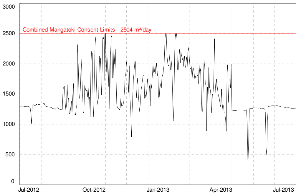
Figure 7 Graph of the daily combined abstraction from the Mangatoki Stream for the Inaha water supply
