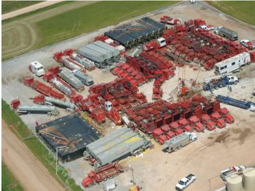
Photo 4 USA wellsite showing typical shale hydraulic fracture wellsite layout around the wellhead (Source: Boeren, 2011)
