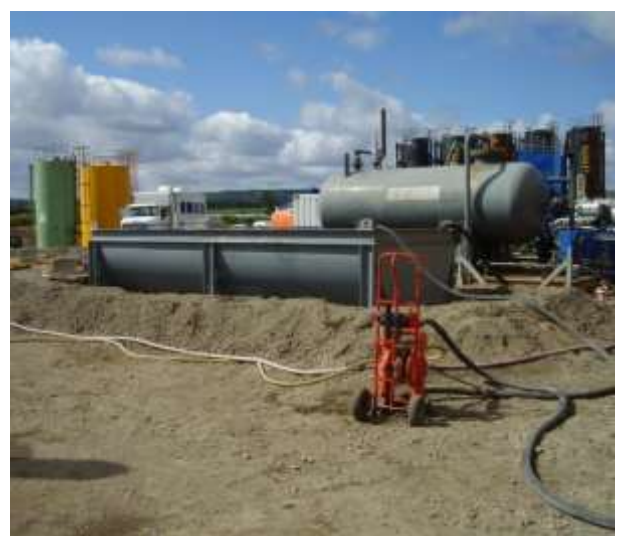
Photo 6 Equipment used in fracture operations at a Taranaki wellsite – pumping equipment, liquid storage, and separator vessel and overflow trough
