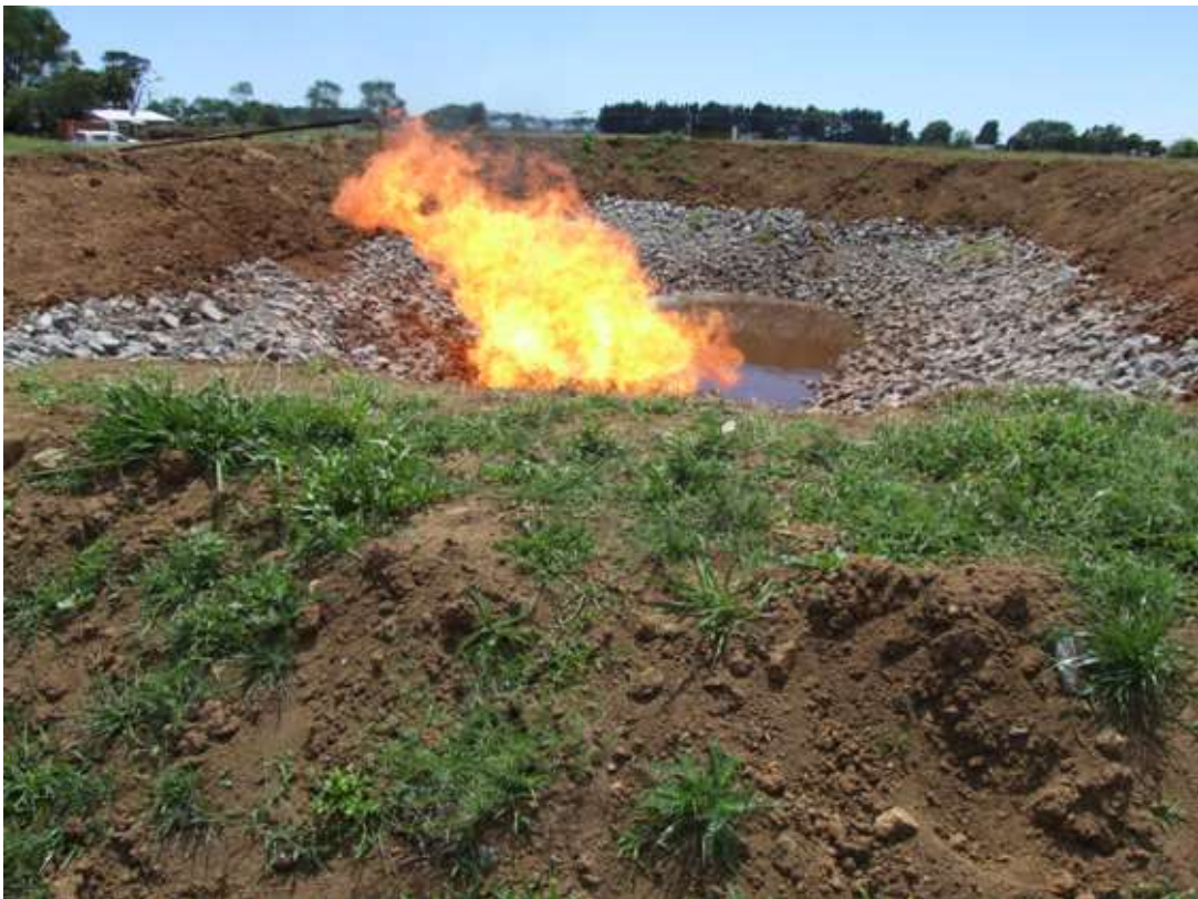
Photo 8 Lined flare pit with fracture fluids being flared and air quality sampling occurring as reported in this report (section 4.8.3)
