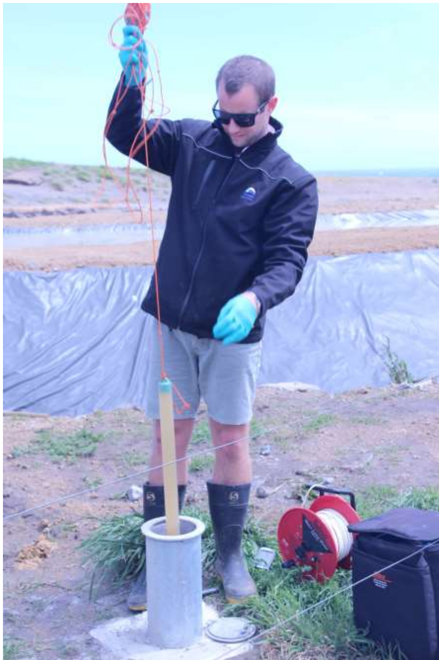
Photo 9 Oeo land farm – lined waste storage pits and groundwater sampling
