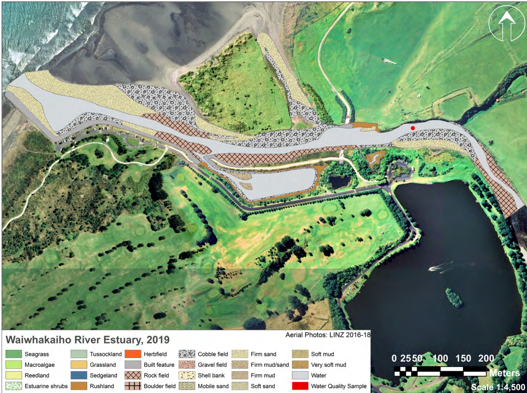
Figure 10. Distribution of intertidal substrata, macrophyte and saltmarsh, and water quality sampling locations, Waiwhakaiho River Estuary, 2019. Water quality sampling involved assessment of conditions in both surface (0.2m) and bottom (0.5m from bottom) waters at each site.
