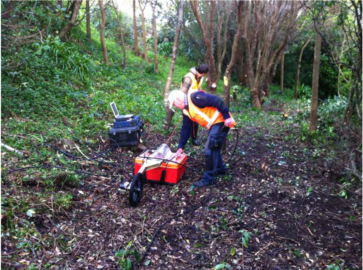
Figure B2 – Collection of GPR data at the Moturoa-3 site.
