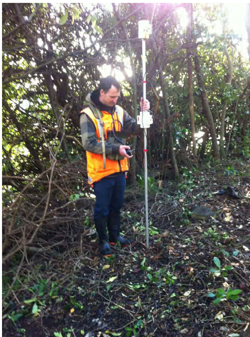
Figure B1 – Collection of magnetometer data at the Moturoa-3 site.
