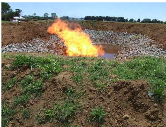
Figure 1 Flaring of natural gas above fracture fluids (water-based with volatile compounds)
