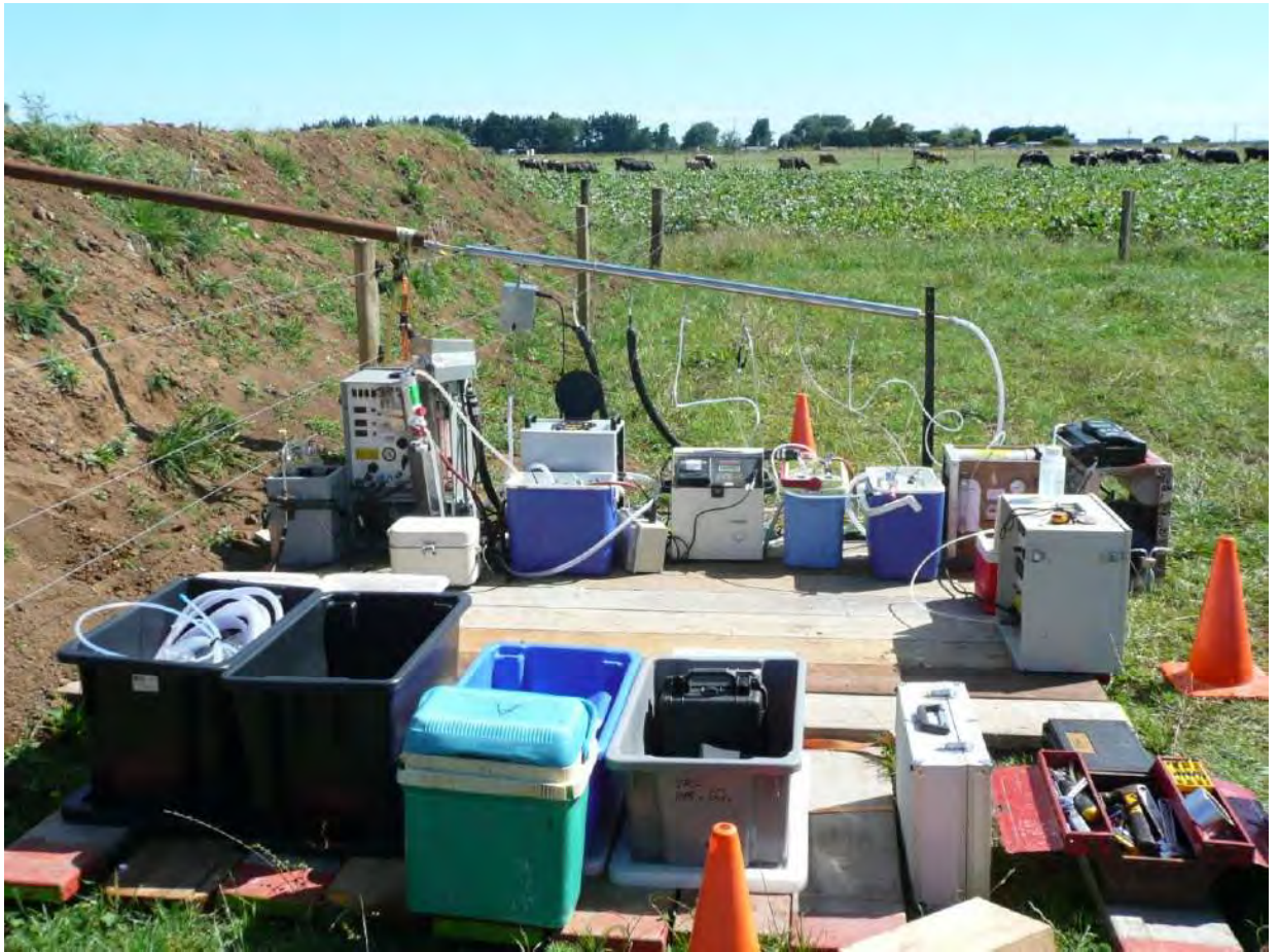
■ Figure 4: Sampling Manifold with Sampling Trains Attached
