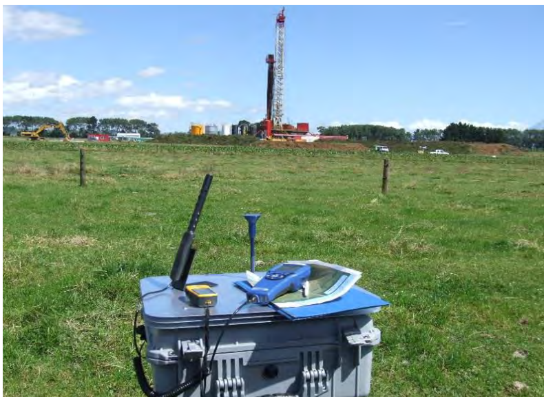
Figure 3 DustTrak and Q-Trak set up at Site (e)
