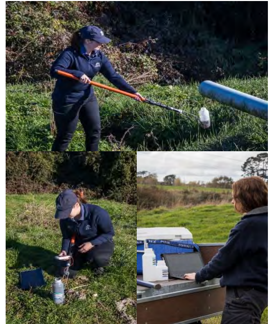
Photo 4 Collecting samples, recording temperature and entering sample information into the laboratory database remotely
