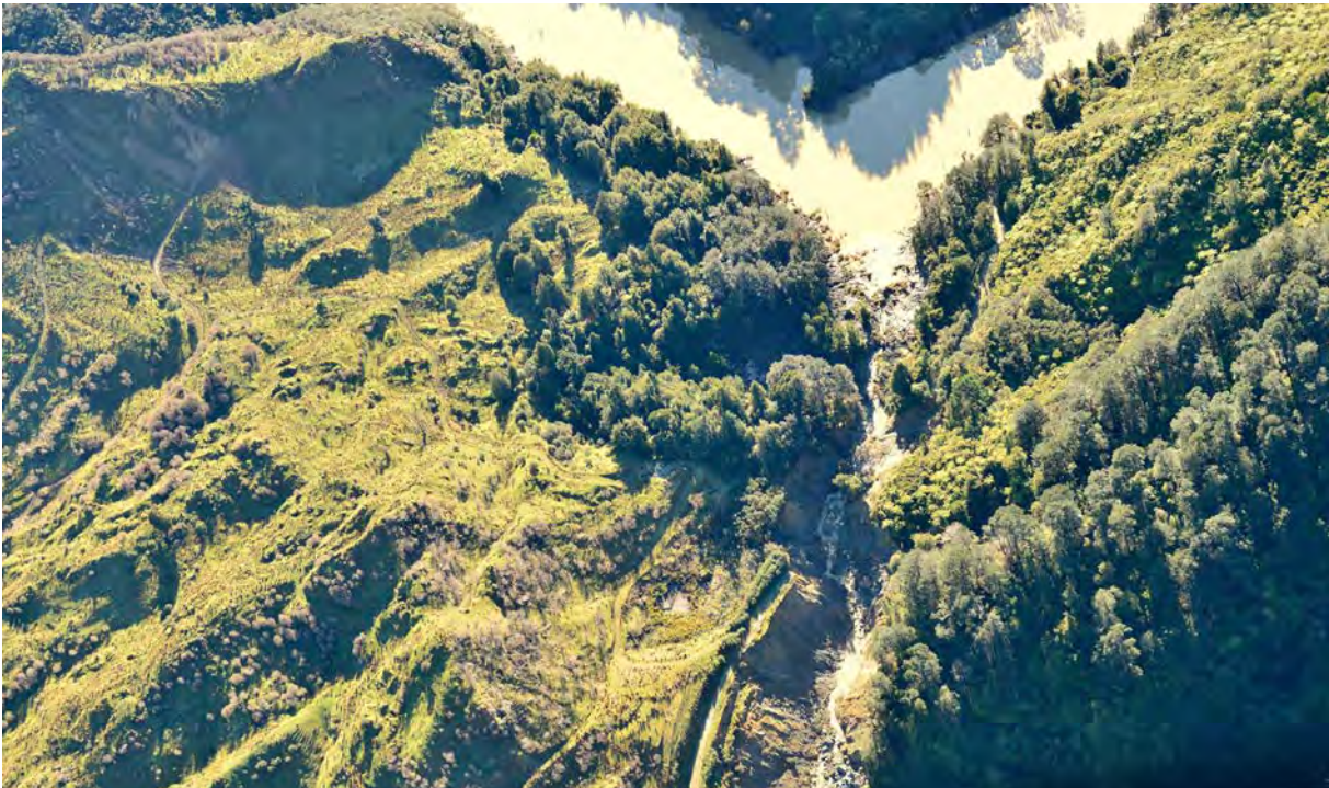
Figure 55 Outlet channel of Lake Mangawhio showing incision that occurred during June 2015 storm. Note location of the county road, and the point where it crossed the outlet channel. (GNS Photo: D02_1420)
