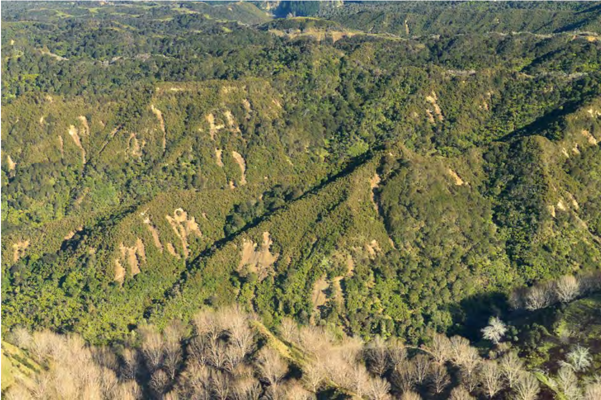
Figure 18 Moderate landsliding in scrub underlain by Pliocene sandstone, 5 km north of Parikino, on western side of the Whanganui River. (GNS Photo: D02_1211)
