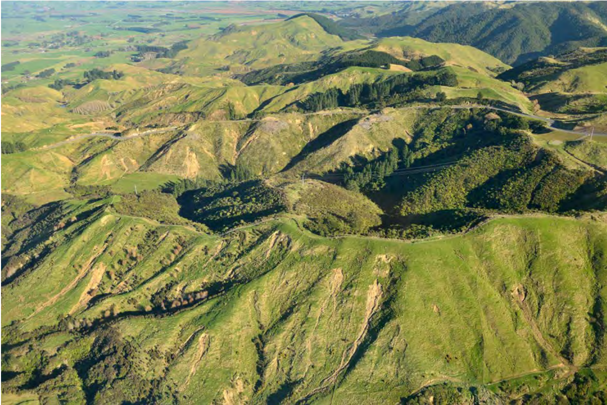
Figure 34 Moderate landsliding on mudstone near Saddle Rd, north of Manawatu Gorge. (GNS Photo: D02_1872)
