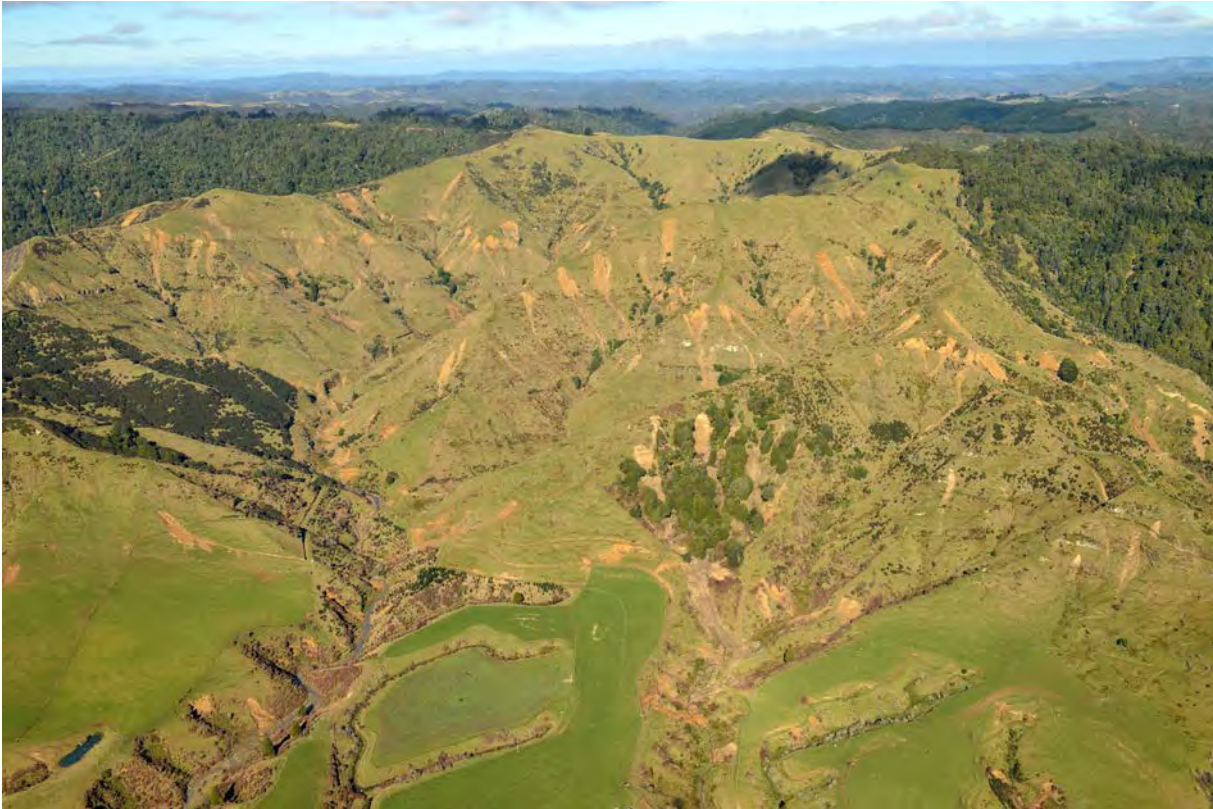
Figure 42 Moderate landsliding in the Mangaehu Stream catchment on Miocene age Whangamomona Group Sandstone. (GNS Photo: D02_2758)
