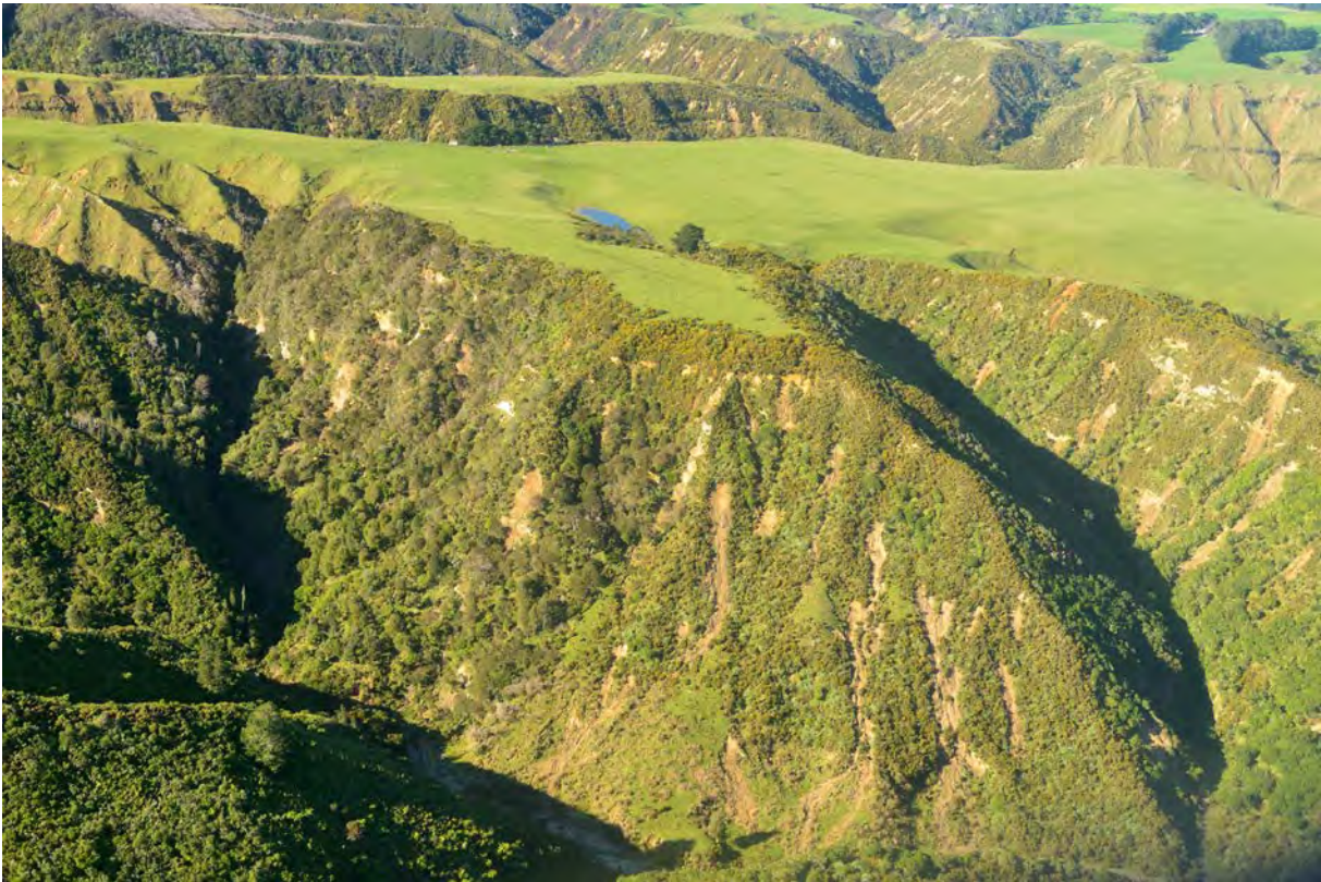
Figure 19 Moderate landsliding in scrub on Whenuakura Group sandstone, near Ridge Rd north of Ngutuwera, Waitotara catchment. (GNS Photo: D02_1370)
