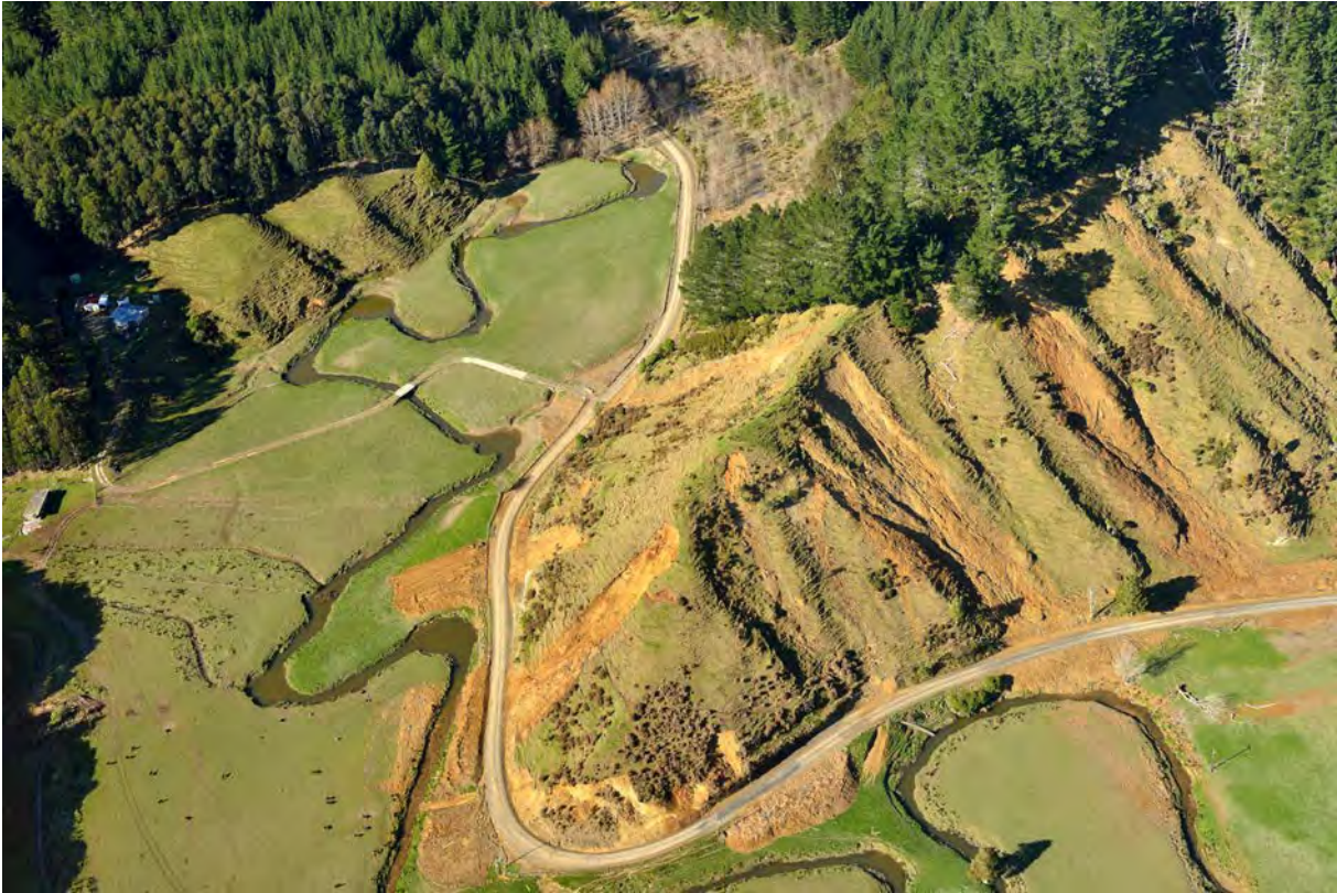
Figure 44 Localised severe landsliding near Uruti, on Miocene age Mt Messenger Formation sandstone, Whangamomona Group. (GNS Photo D02_2579)
