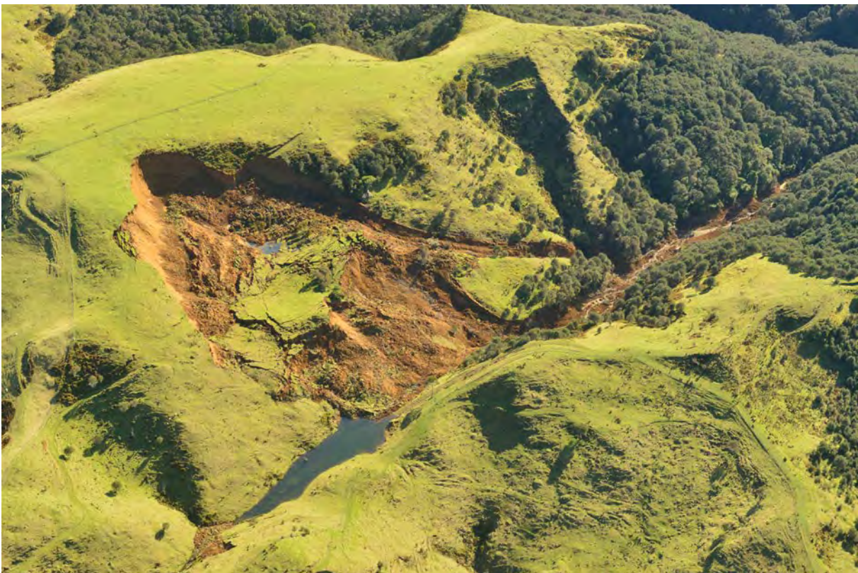
Figure 47 Deep-seated landslide near Pohokura saddle, Waitara River, on Miocene age Whangamomona Group sandstone (Kiore Formation). Note the small lake formed upstream of the landslide debris. (GNS Photo: D02_2620)
