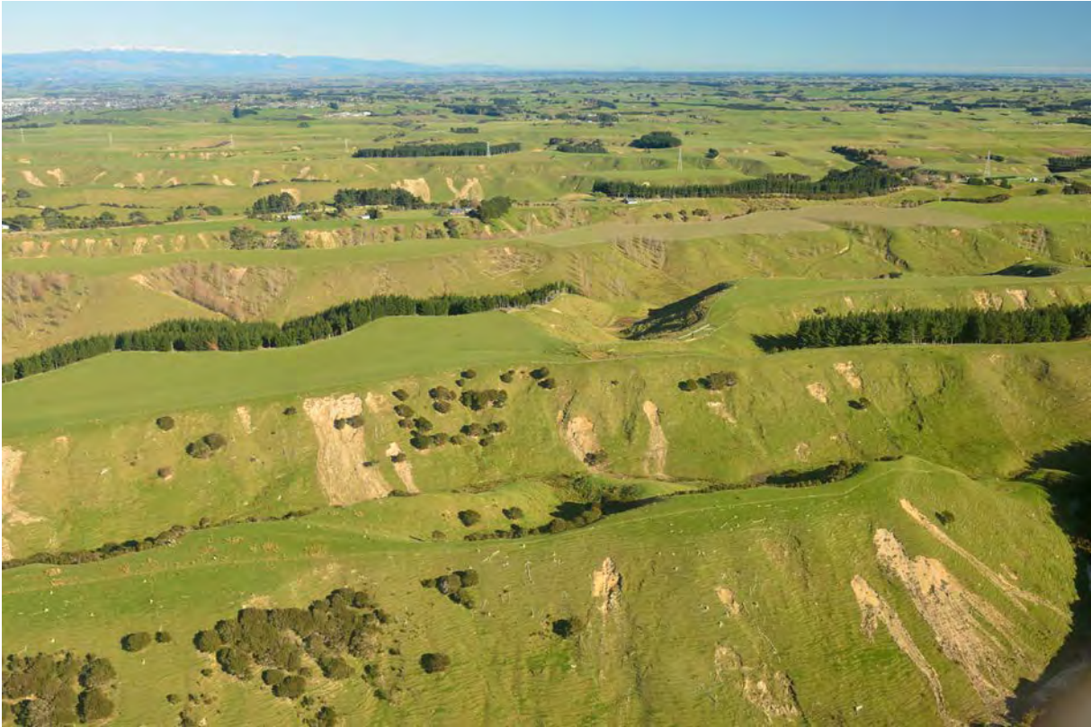
Figure 5 Moderate landsliding on Shakespeare Group (Quaternary) marine sediments, 6 km east of Halcombe (north-facing slopes). (GNS Photo: D02_1840)
