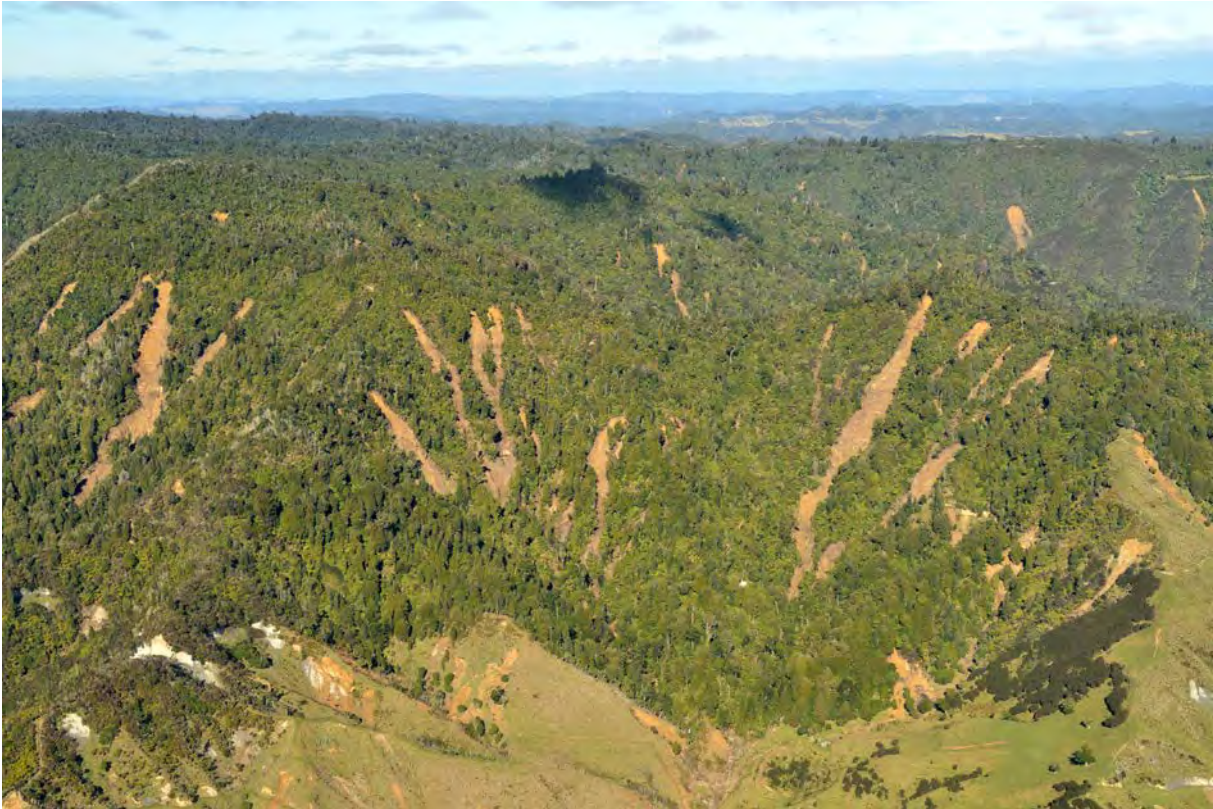
Figure 37 Landslides on mature indigenous forest covered slopes in the Puniwhakau Stream catchment, a tributary to the Mangaehu Stream, Matemateaonga Range near Tututawa. Whangamomona Group sandstone. (GNS Photo: D02_2767)
