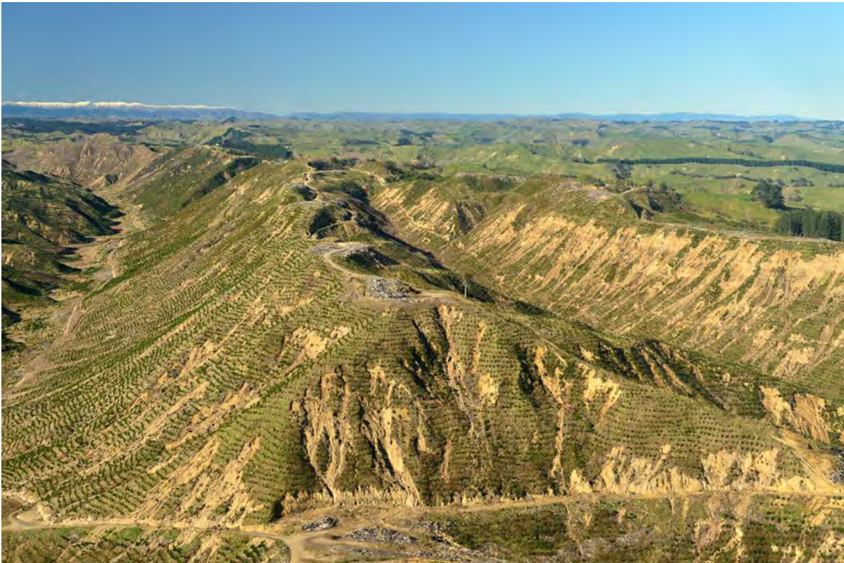
Figure 17 Severe landsliding in areas of new plantings on Maxwell Group sandstone, Matariki Forest, Whangaehu Valley. (GNS Photo: D02_1596)
