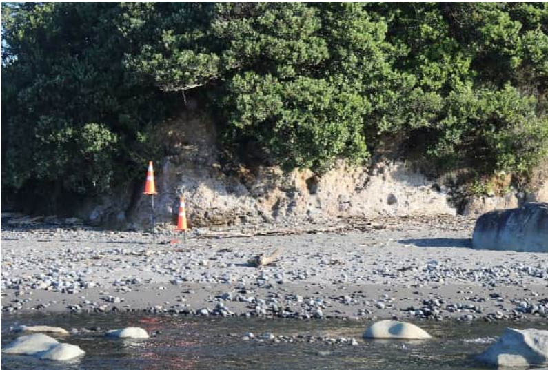
Figure 19 Photograph showing the surveyed points where height has been determined. The proposed RL of the rock revetment that has been designed is located at the bottom of the top white line on the lower cone.
