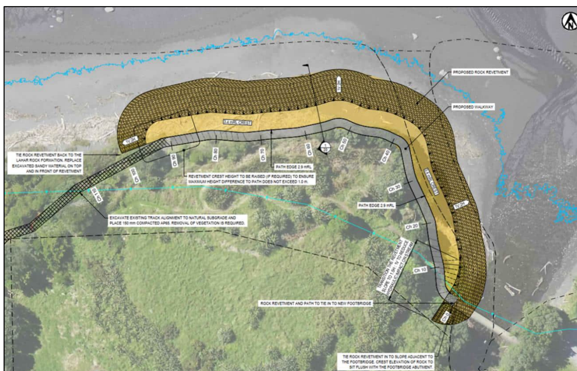
Figure 1.4: Concept design for the rock revetment and pathway installation around Weld Road Reserve headland and the extent of works within the coastal marine area (CMA).
