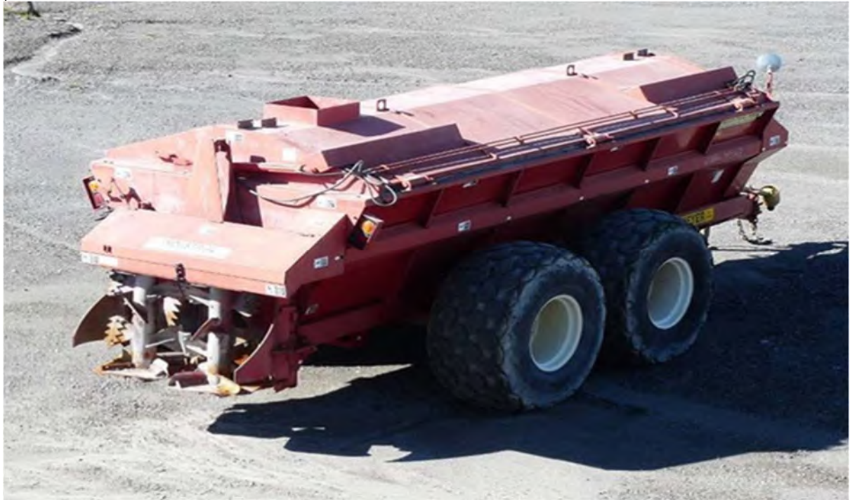
Photo 1 Spreader used for dispersing drilling waste over the landfarming area.
