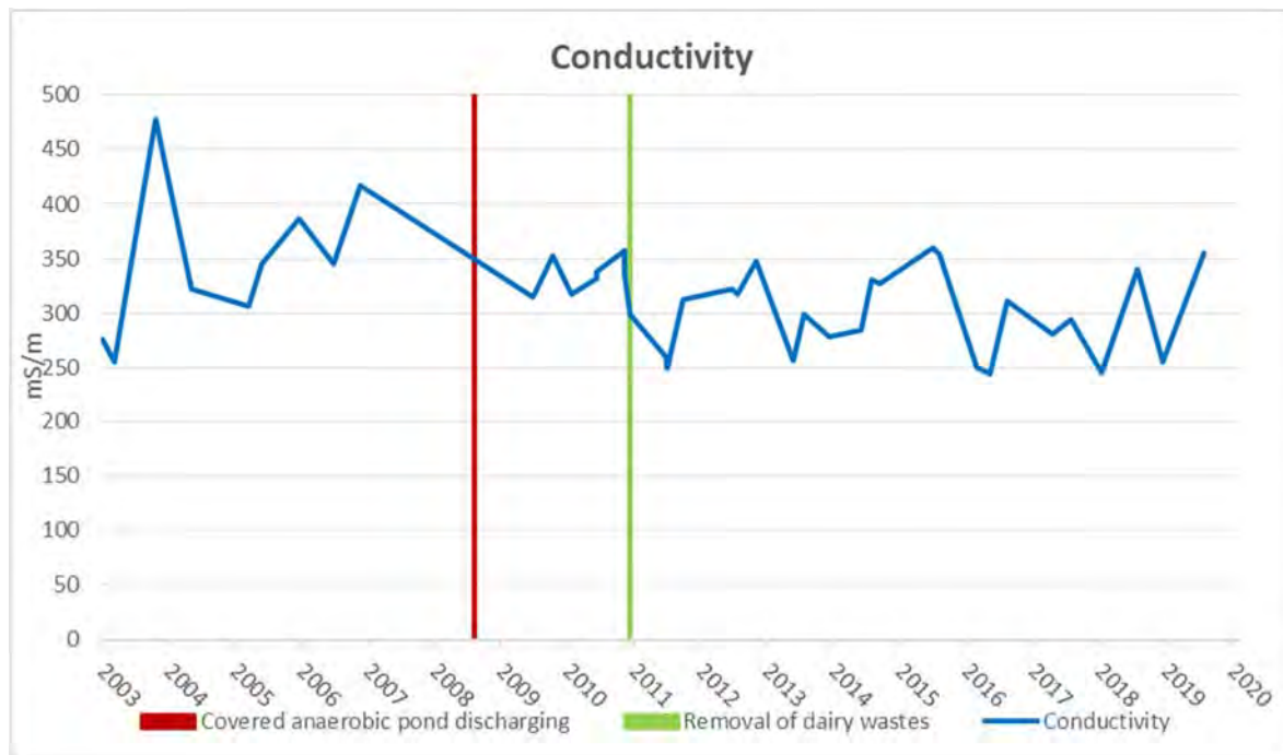
Figure 5 Wastewater conductivity measurements mS/m 2003-2019 at 25°C
