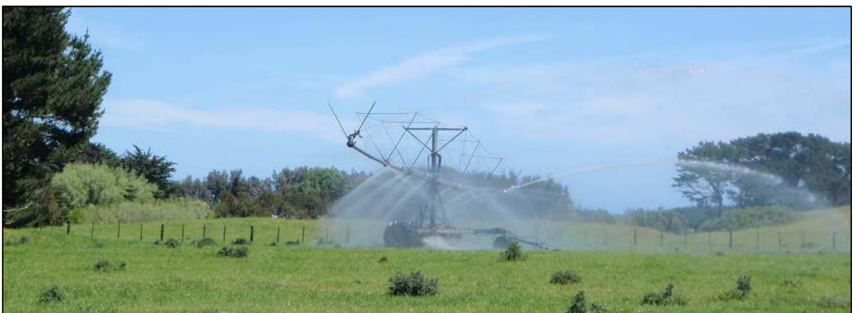
Photo 3 Picture depicting travelling irrigator system
