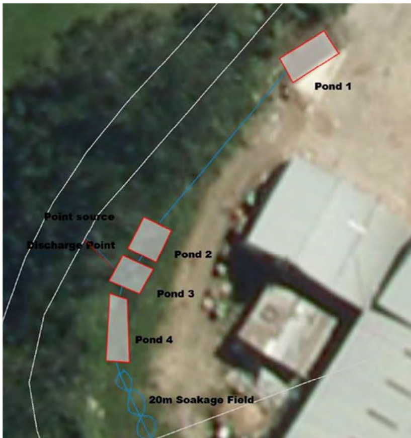
Figure 4 Osflo soakage pond setup
