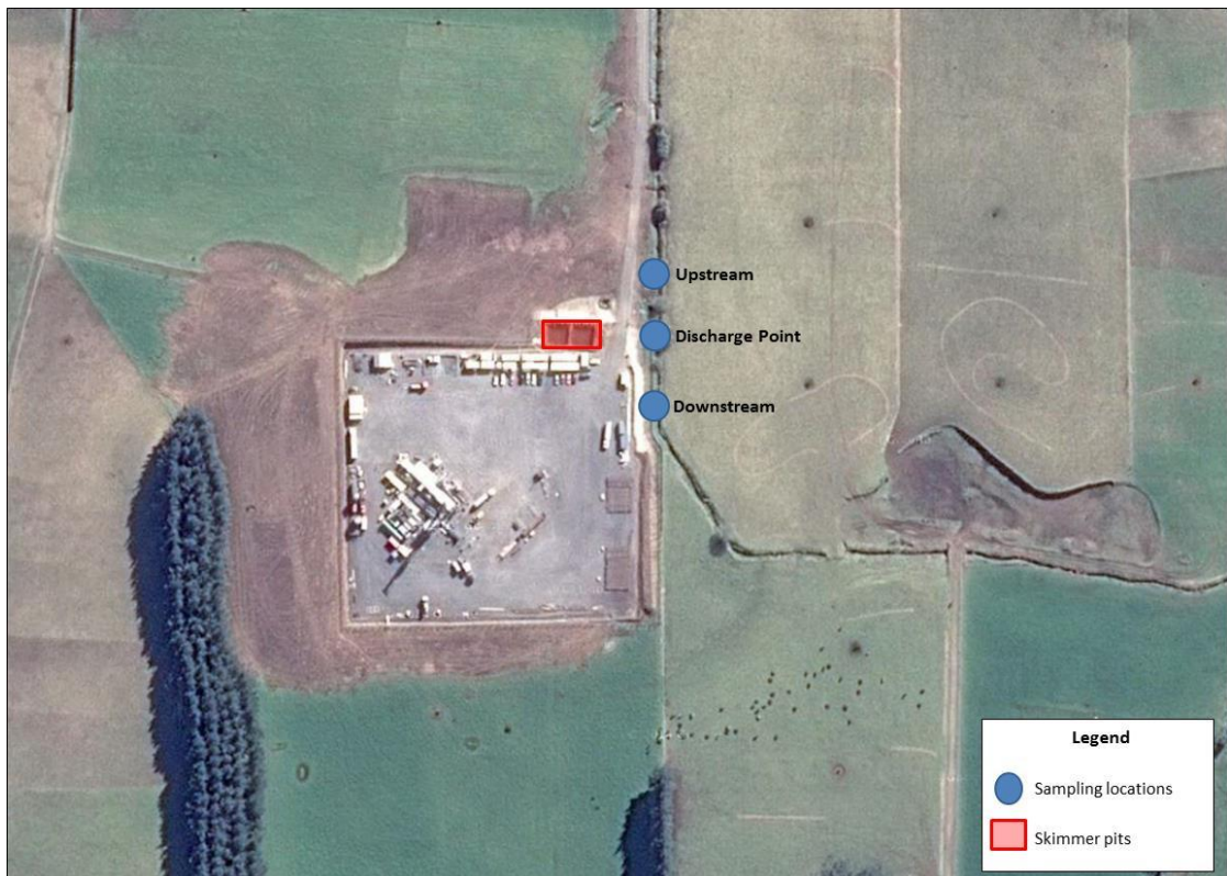
Figure 2 Stormwater and surface water sampling locations at the Cheal-E wellsite
