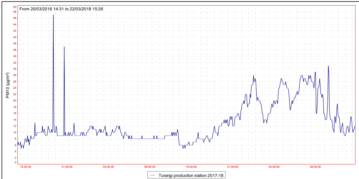
Figure 2 PM10 concentrations ( \mu\text{g}/\text{m}^3 ) at the Turangi production station (2017-18)
