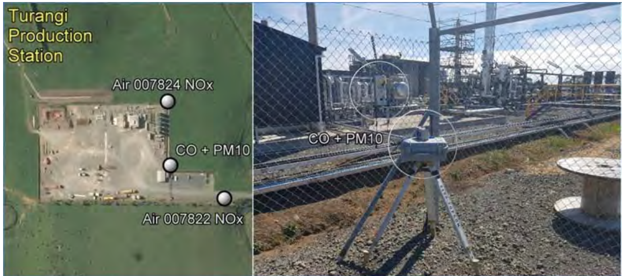
Figure 1 Air monitoring sites at Turangi Production Station for 2017-2018
