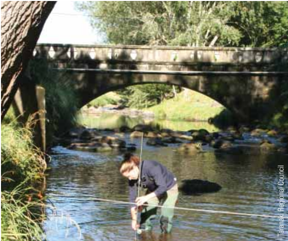
Gauging the flow of the Mangaoraka Stream.
