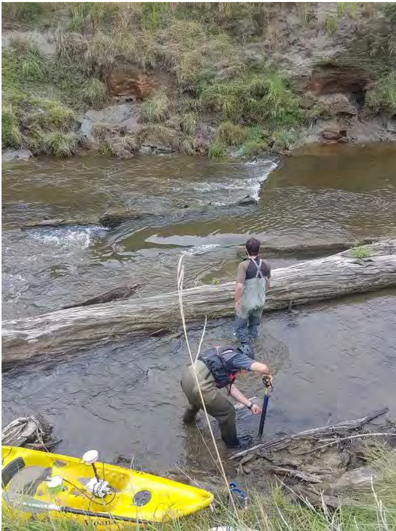
Figure 5: Cross-section 5 on Whenuakura River at flow of about 1.9 \text{ m}^3/\text{s} (above) and flow of 2.4 \text{ m}^3/\text{s} (below).
