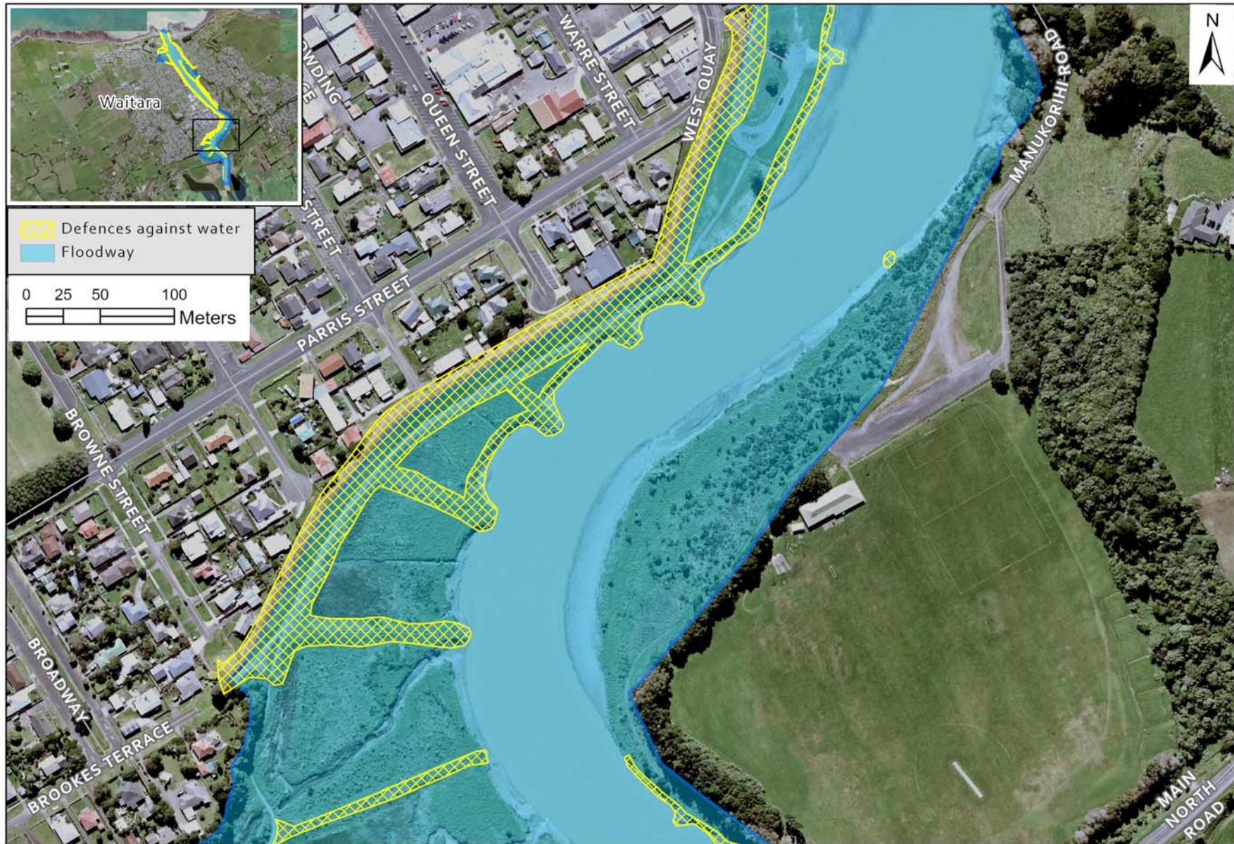
Map 2d Defences against water and floodways along the Waitara River, New Plymouth.
