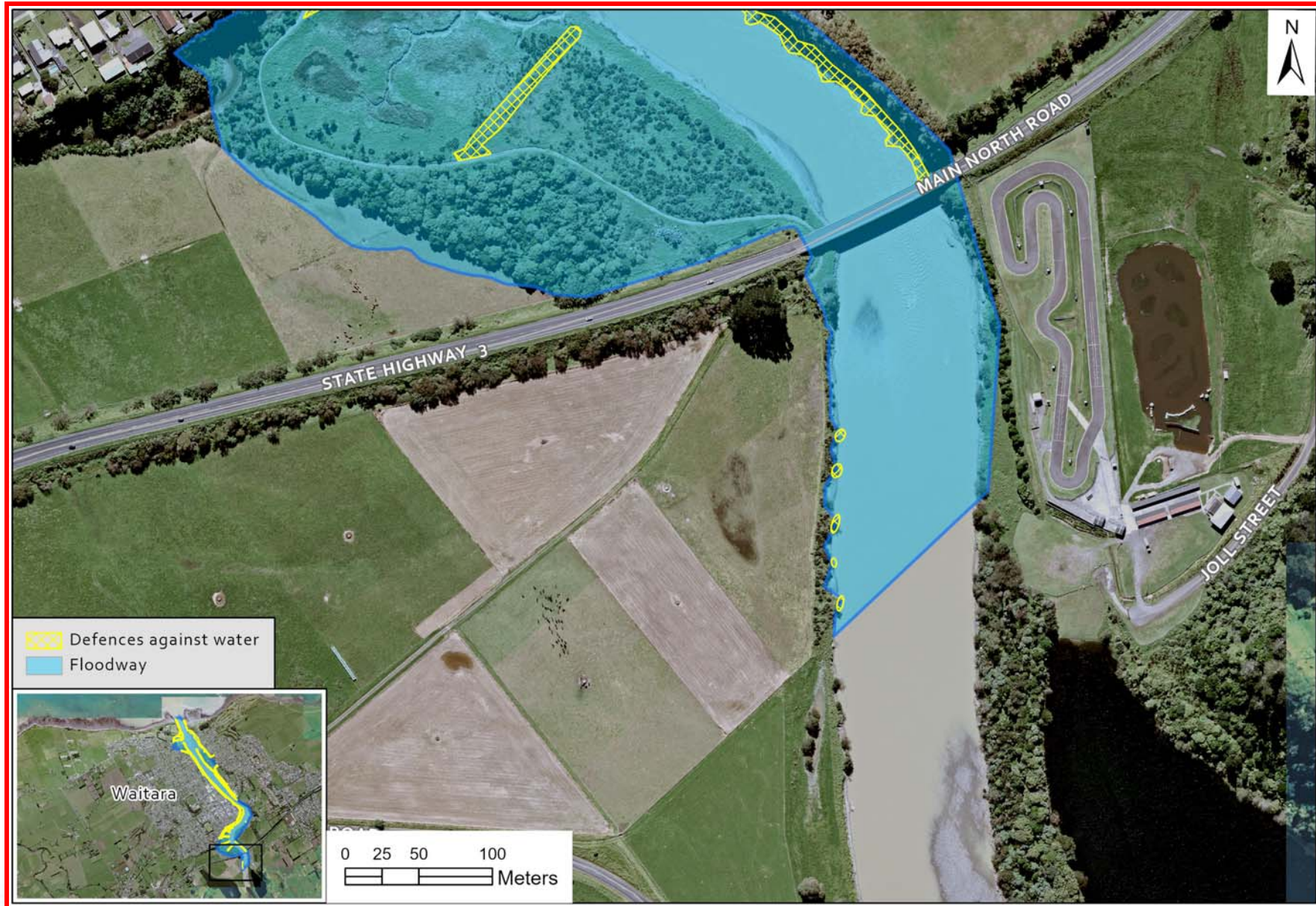
Map 2e Defences against water and floodways along the Waitara River, New Plymouth.
