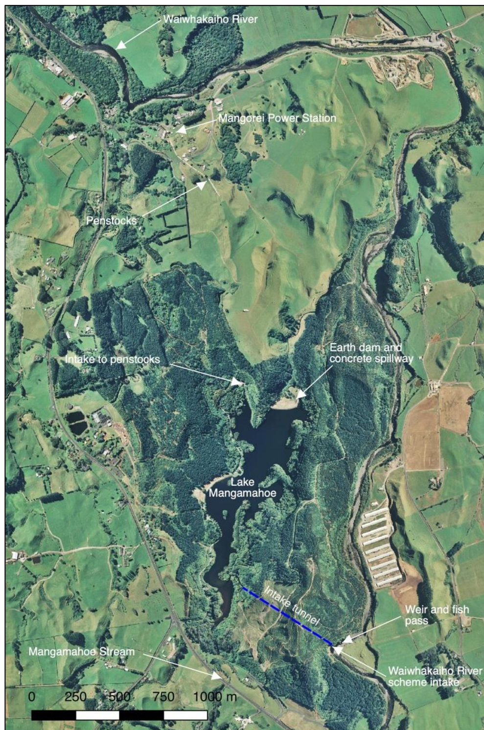
Figure 1. Aerial showing location of structures and surface waters associated with the Mangorei HEPS.
