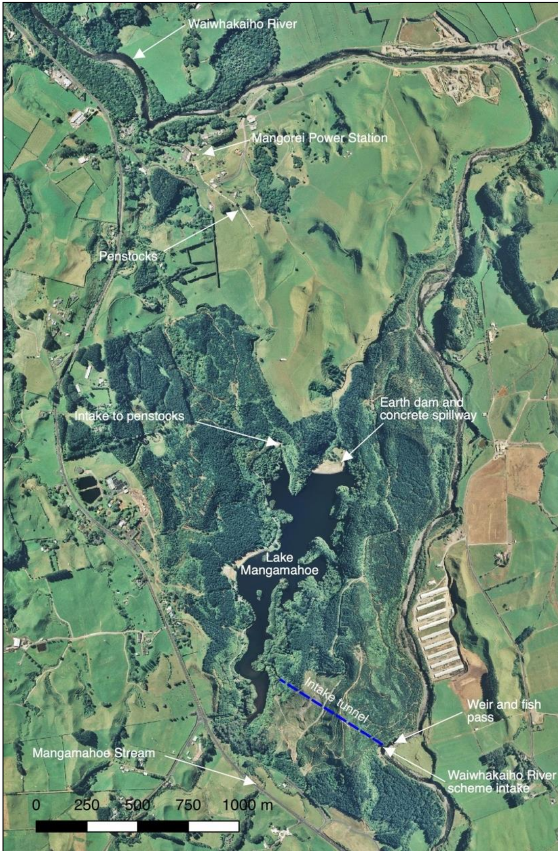
Figure 1. Aerial map showing location of structures and surface waters associated with the Mangorei HEPS.
