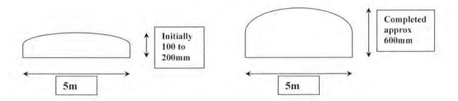
The process involves an extended period of standard aerobic composting conditions over a minimum of 35-40 days. The temperatures for worm processing are a lot lower than that of Greenwaste composting and should range between  $20^{\circ} - 30^{\circ}$  Celsius. The process is
