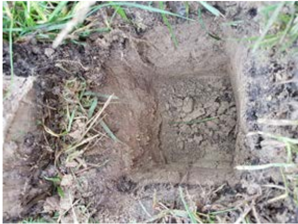
Figure 17. Photo showing soil test pit.
