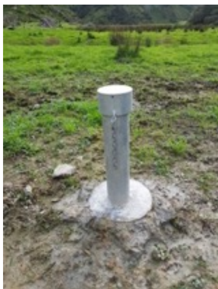
Figure 30. Recently installed groundwater monitoring bore.
