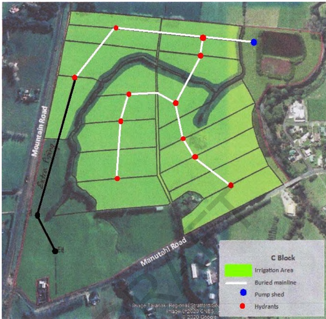
Figure 11 Piping and hydrants locations of the bottom block with current and proposed piping extension
