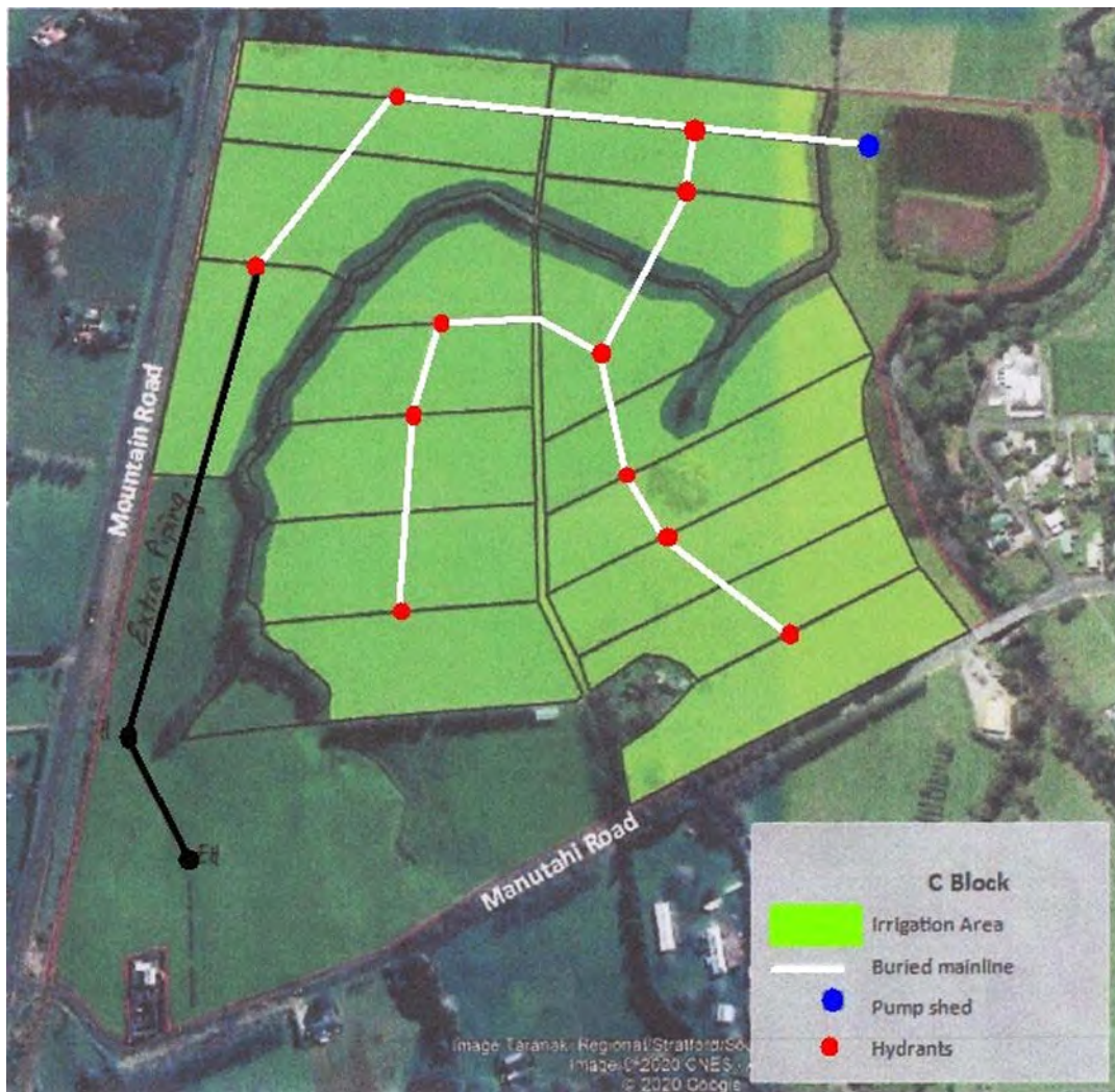
Figure 13 Piping and hydrants locations of the bottom block with current and proposed piping extension
