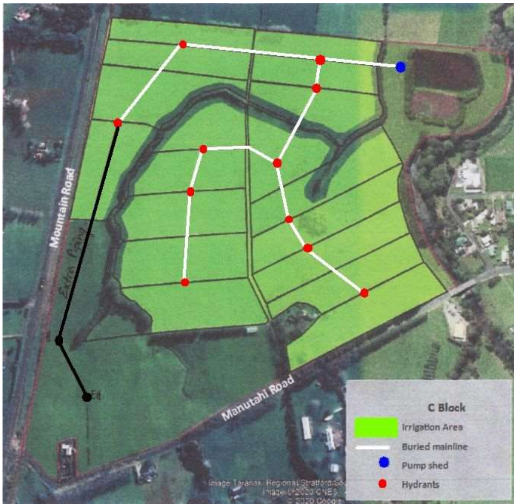
Figure 10 Piping and hydrants locations of the bottom block with current and proposed piping extension
