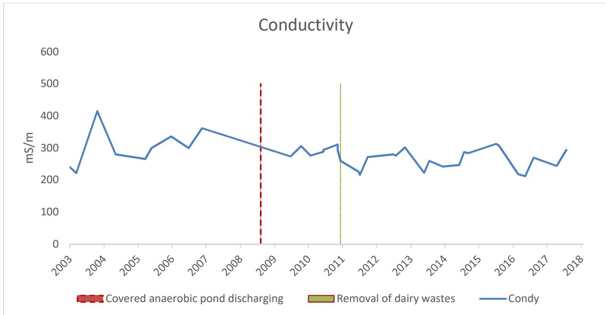
Figure 4 Wastewater conductivity measurements mS/m 2003-2018
