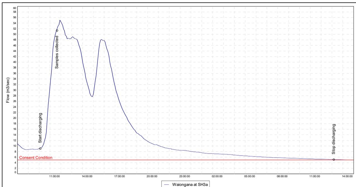
Figure 9 Flow data recorded for the Waiongana Stream during the discharge of wastewater from Leppers piggery, commencing 18 June 2018 at 1010 hrs and finishing 19 June 2018 at 1315 hrs
