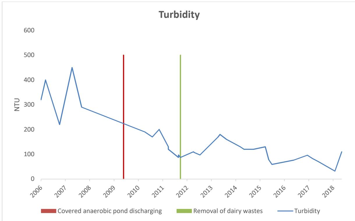
Figure 6 Wastewater turbidity levels, NTU, 2003-2018
