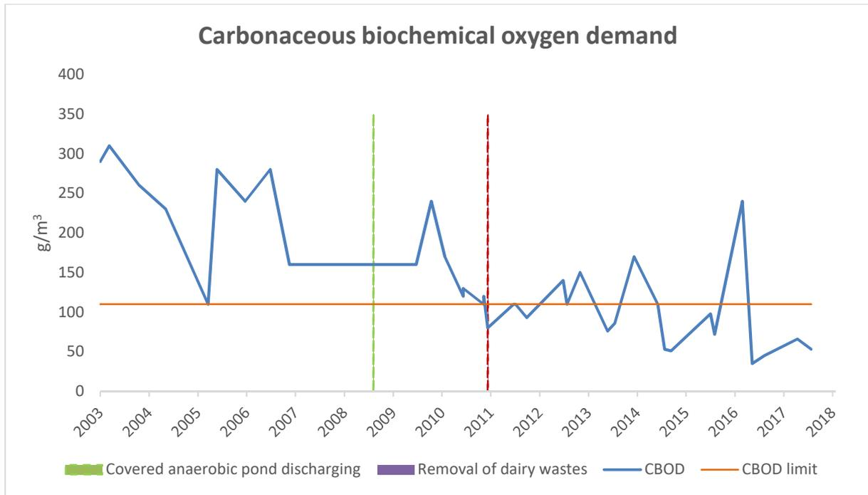
Figure 2 Wastewater carbonaceous biochemical oxygen demand levels, g/m<sup>3</sup>, 2003-2018
