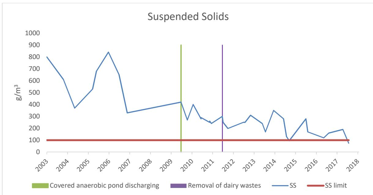
Figure 5 Wastewater suspended solids levels, g/m<sup>3</sup>, 2003-2018
