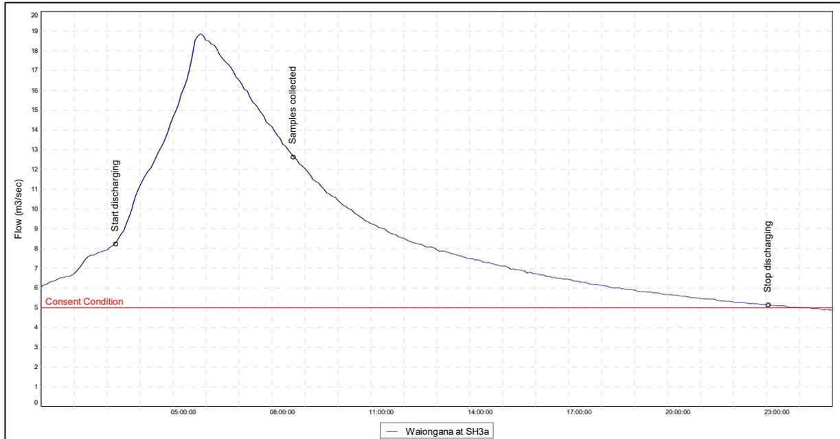
Figure 8 Flow data recorded for the Waiongana Stream during the discharge of wastewater from Leppers piggery, commencing 8 March 2018 at 0300 hrs and finishing 8 March 2018 at 2300 hrs
