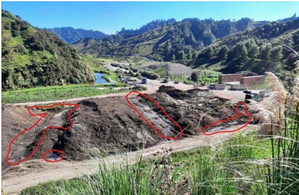
Photo 1 Windrows on Pad 1. Note the height is greater (4 to 5 m) than the maximum recommended by NZS4454 (~2 m) and stagnant wastewater is present in the proximity of the piles (encircled in red). Photograph taken 01/03/2022
