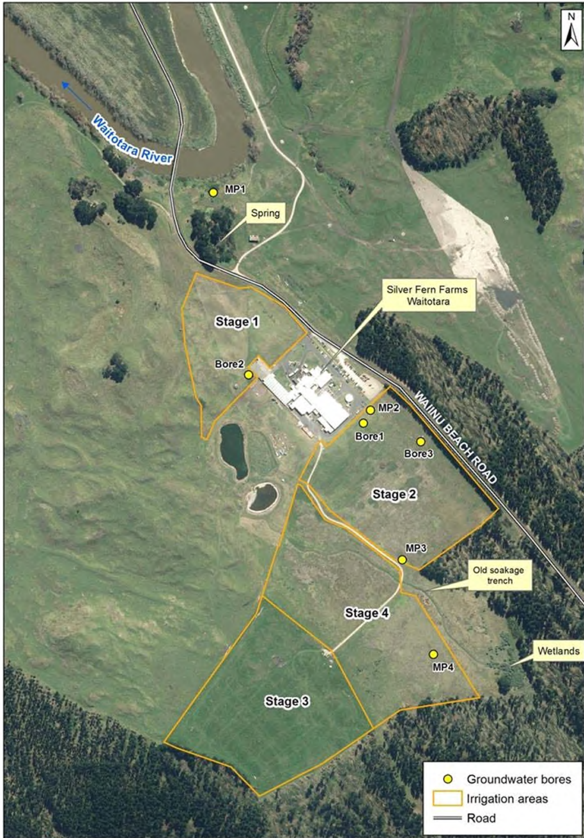
Figure 1 Location of Silver Fern Farms Waitotara meat processing plant showing irrigation areas and groundwater monitoring points
