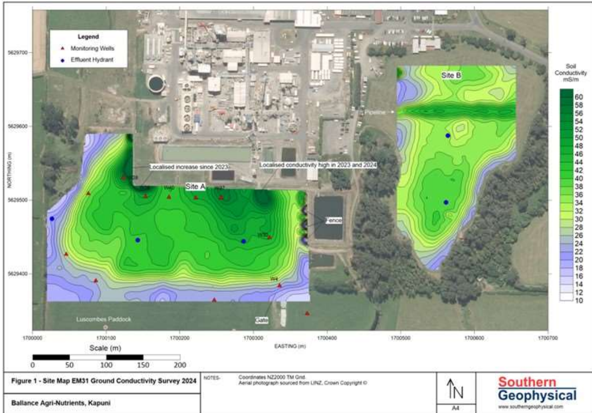
Figure 8 Site Map EM31 Ground Conductivity Survey 2024 (Southern Geophysical 2024)
