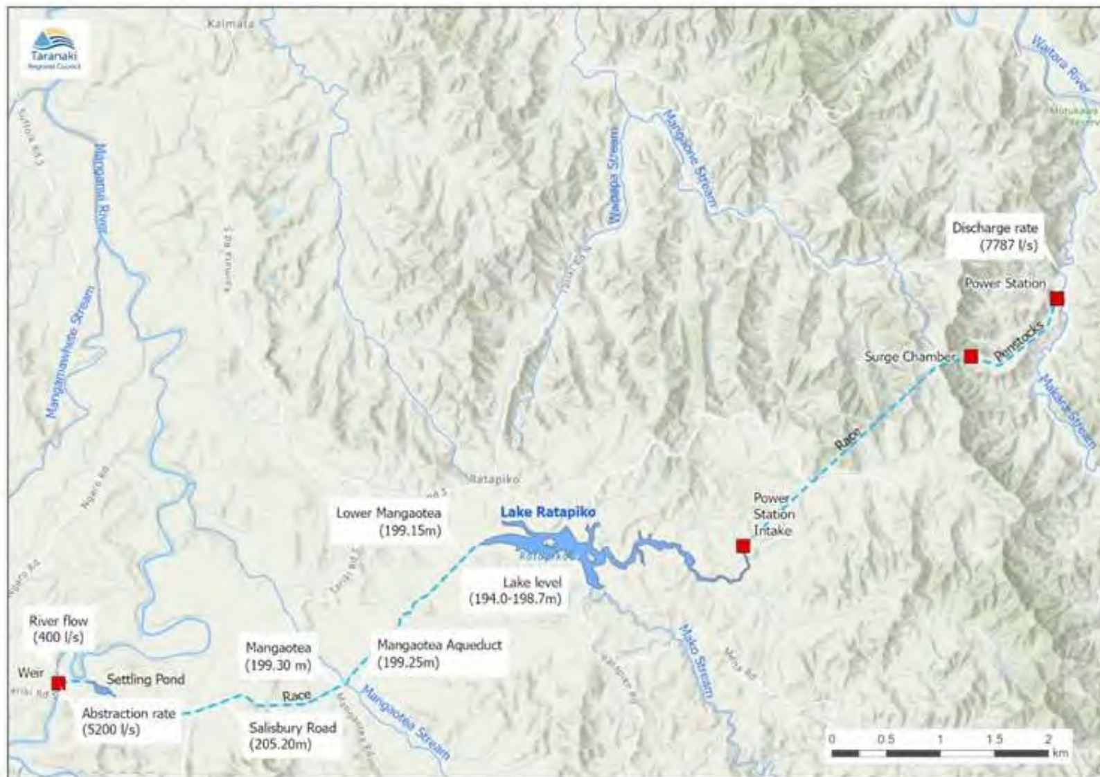
Figure 3 Location of water abstraction, discharge and water level monitoring sites for the Motukawa HEP scheme (limits in brackets)
