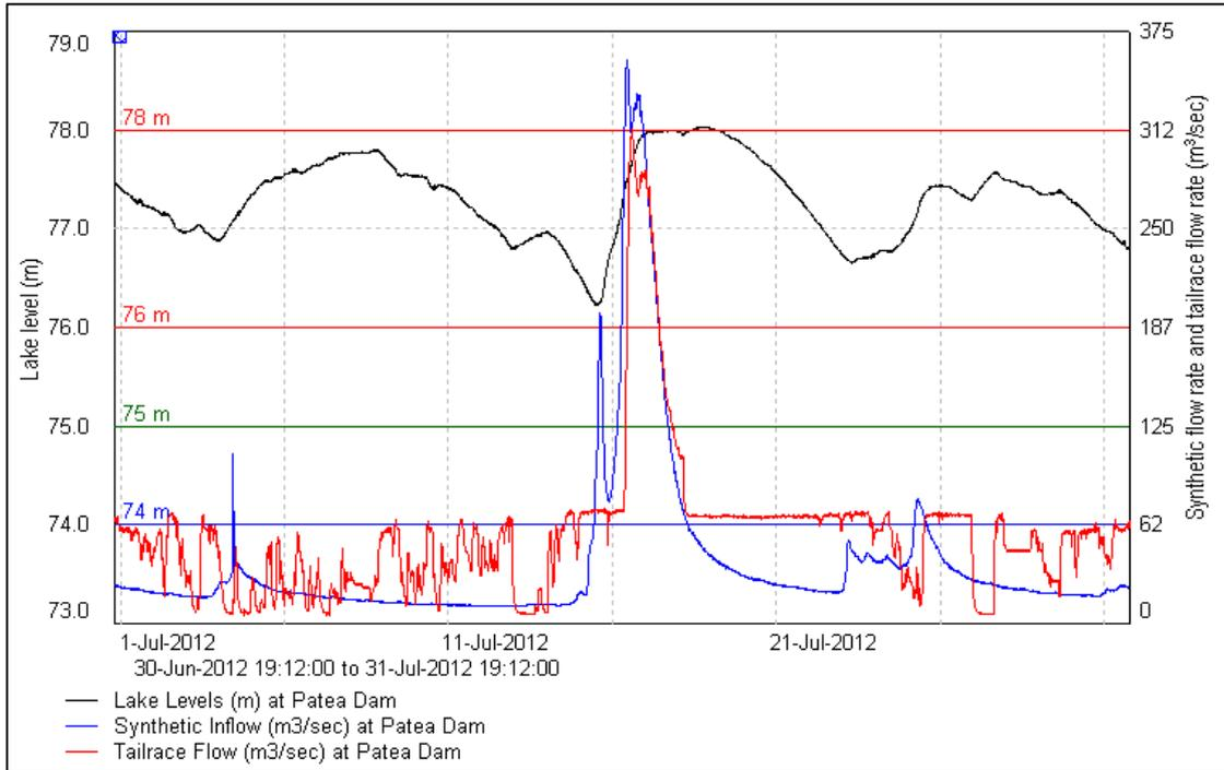
**Figure 6** The relationship between lake levels, inflows and tailrace flows (generation flow plus spill-flow)
