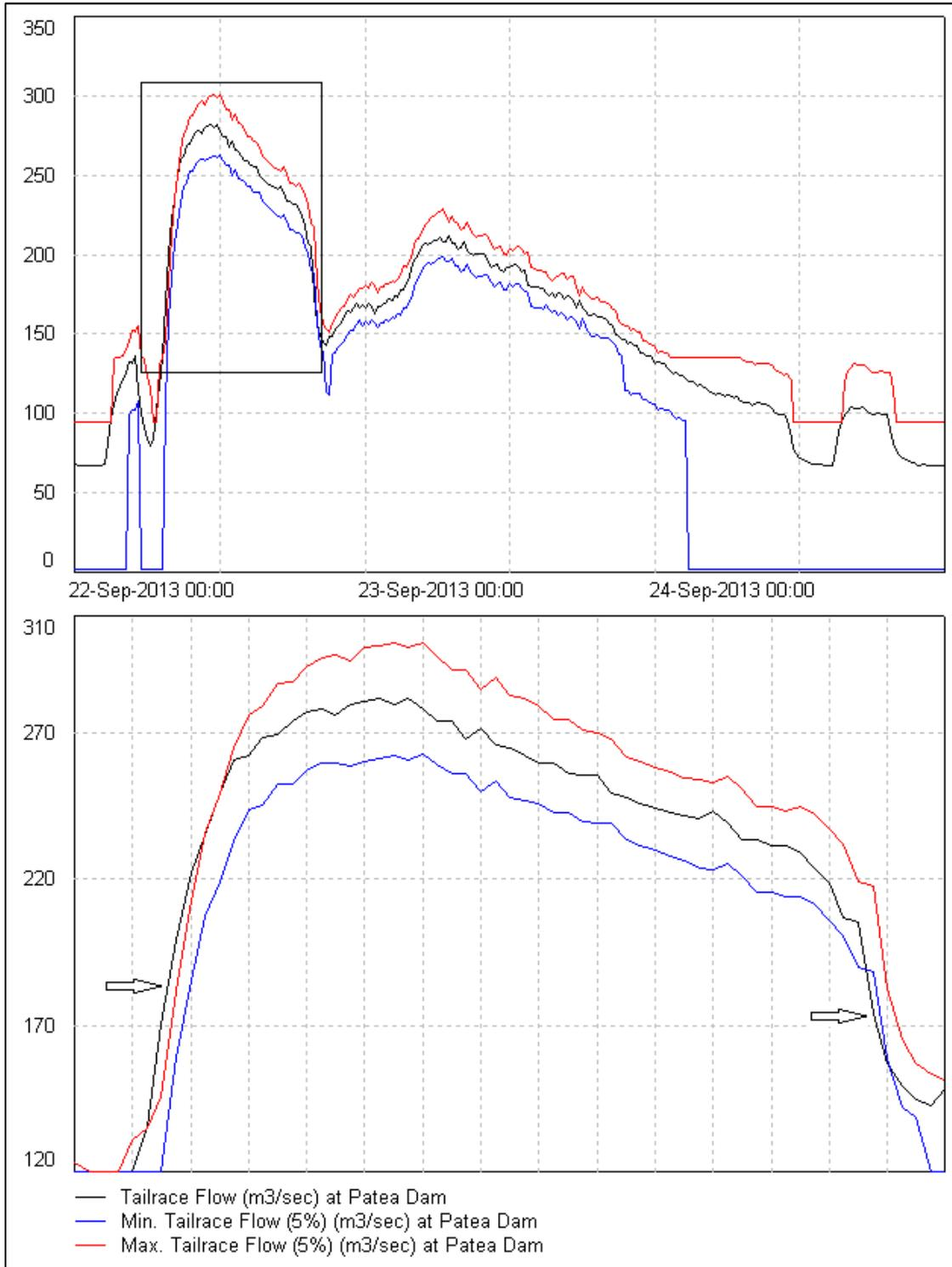
**Figure 3** Tailrace flow from 22 September to 25 September 2013, compared with maximum and minimum allowable tailrace flow.
