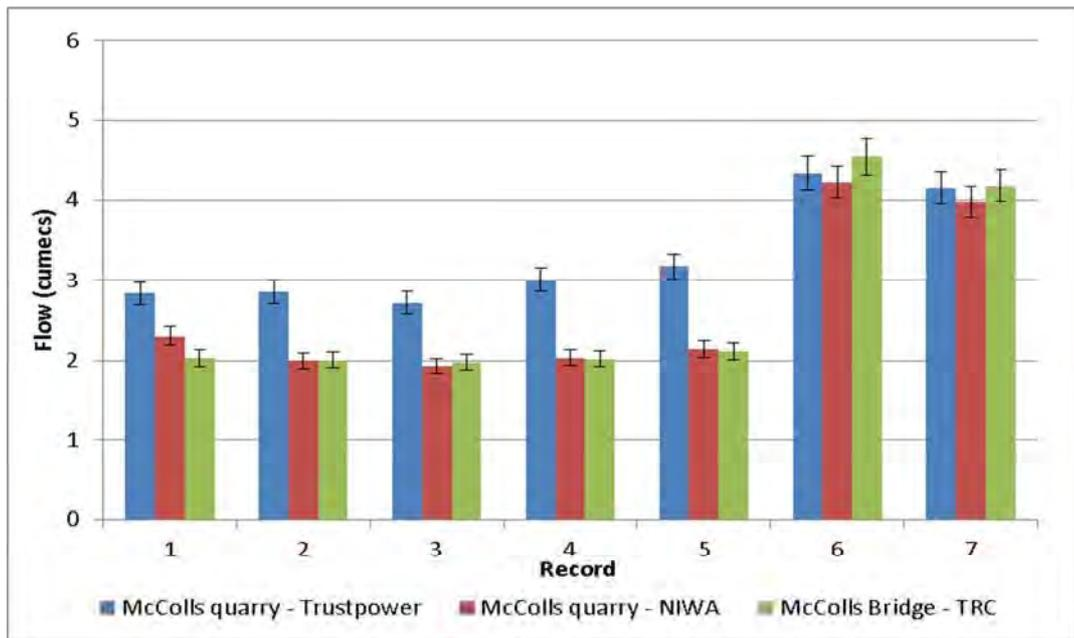
**Figure 8** Average flows recorded at the three recorder stations over seven time periods, including 5% error bars
