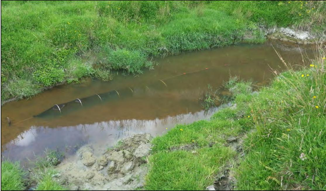
Photo 1 A fyke net, set at site 2, Haehanga Stream.
