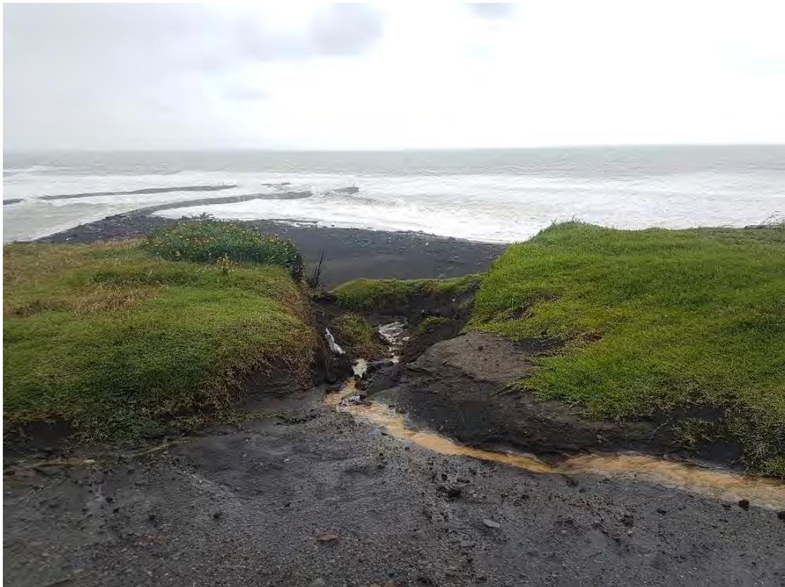
Photo 1 Stormwater erosion in south eastern area of the site 6 December 2018
