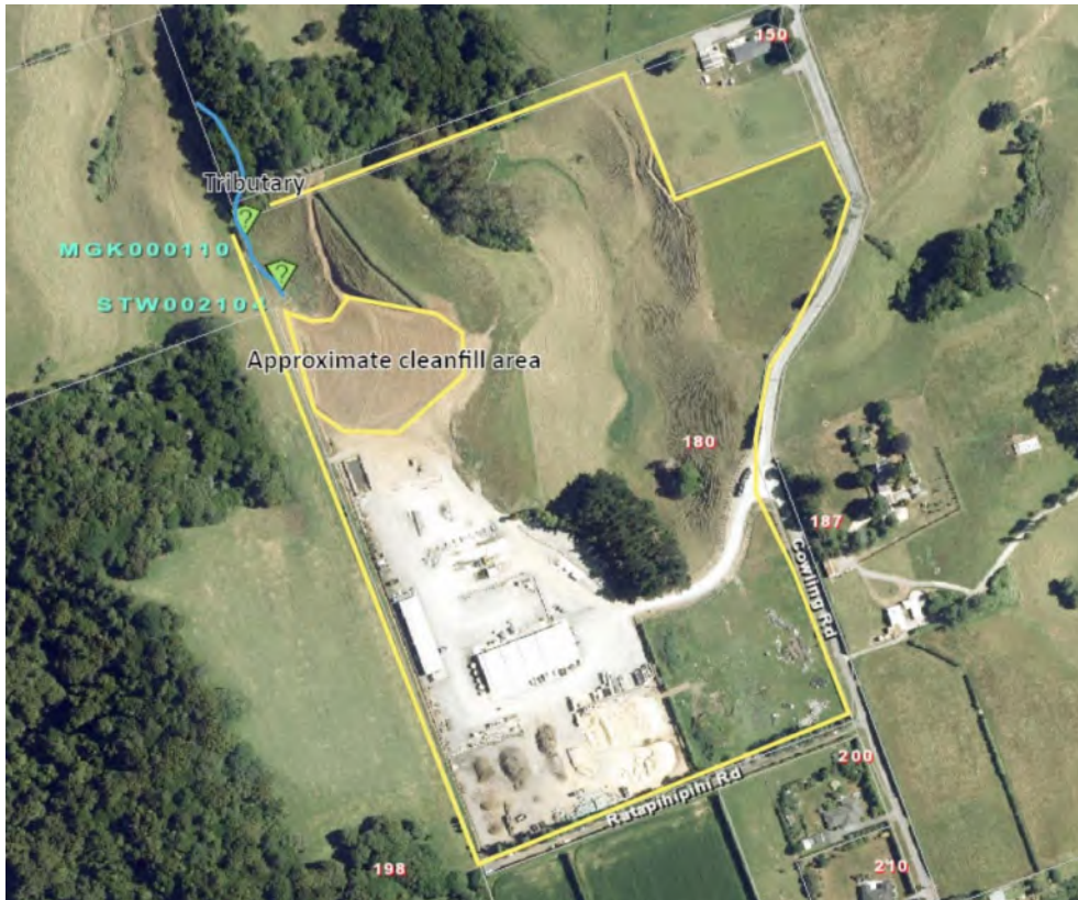
Figure 3 Downstream receiving water (MGK000110) and discharge (STW002104) sampling sites at Westtown Haulage cleanfill. Aerial image from 2021
