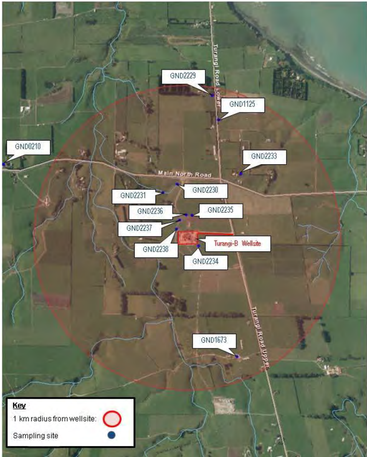
Figure 2 Location of groundwater sampling sites in relation to the Turangi-B well site
