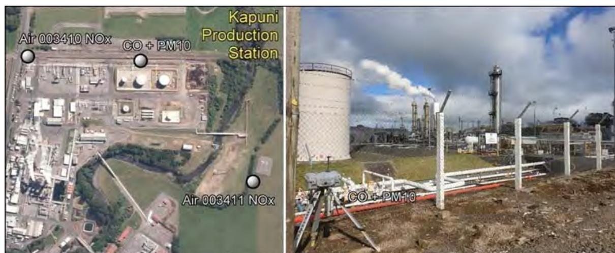
Figure 3 Air monitoring sites at Kapuni Production Station for 2019-2020
