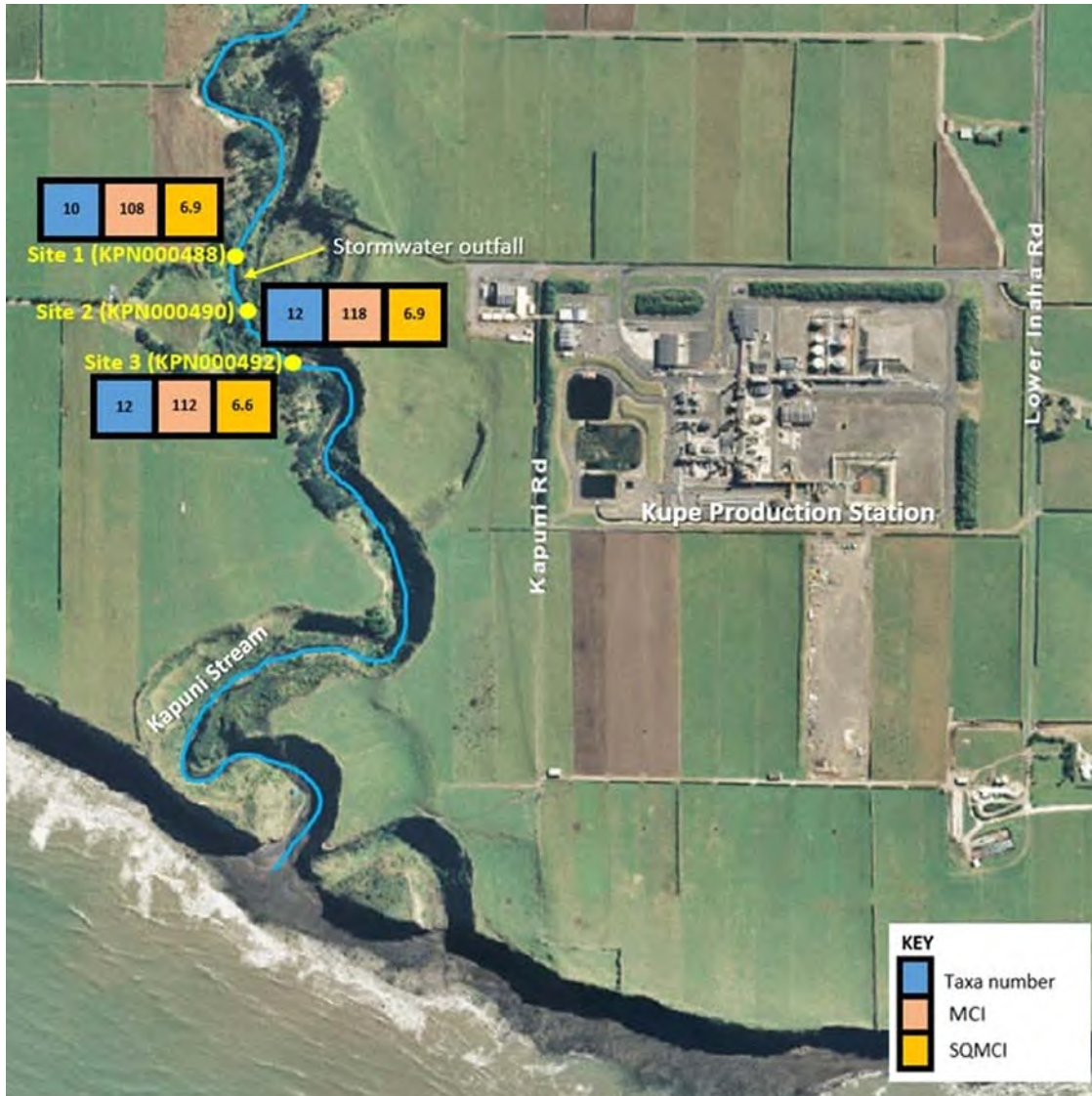
Figure 5 Biomonitoring sites in the Kapuni Stream in relation to the Kupe Production Station, with taxa number, MCI scores and SQMCI scores for each site, spring 2022
