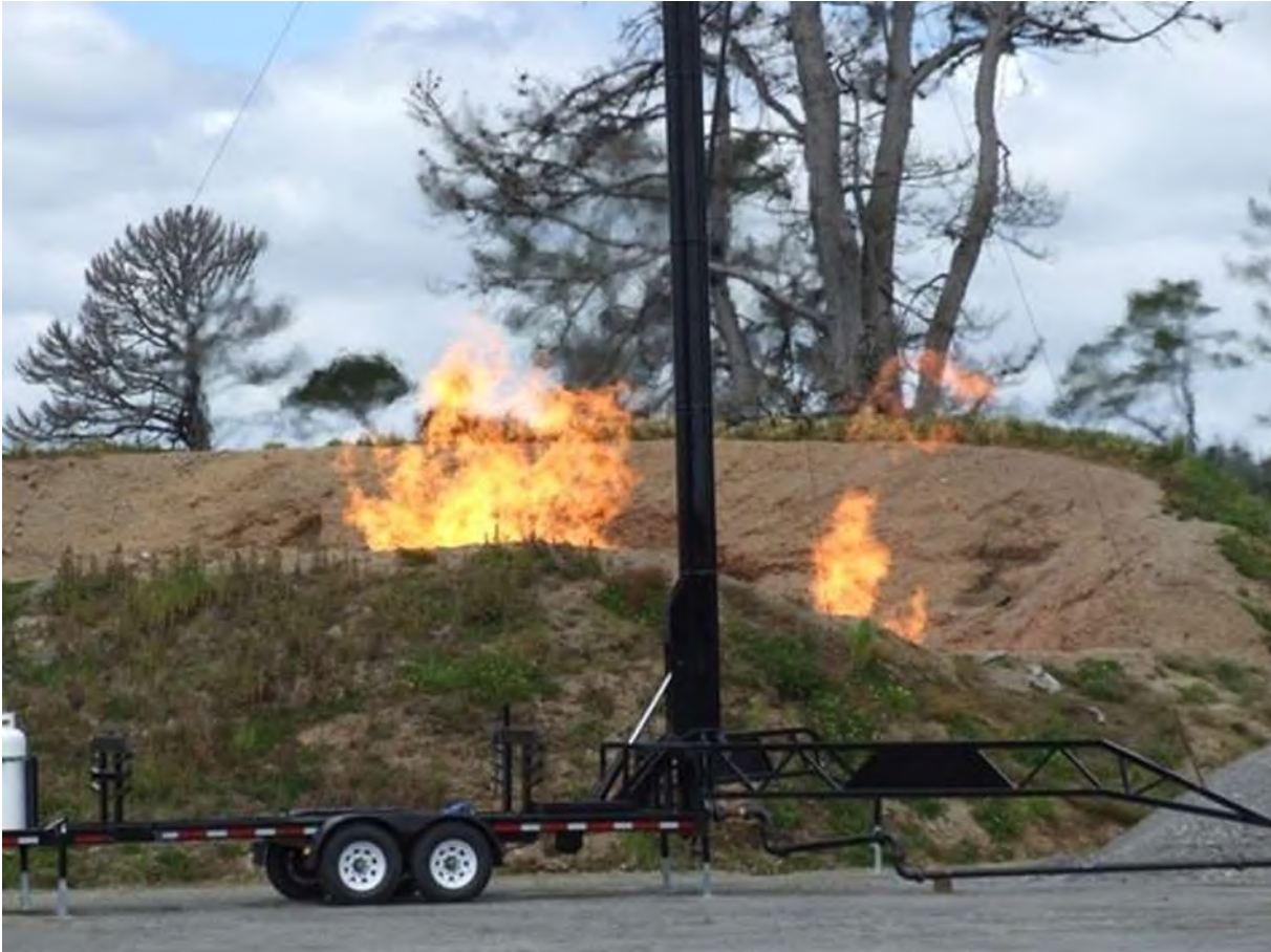
Figure 3 Burning flare in the flare pit at the Sidewinder Production Station
