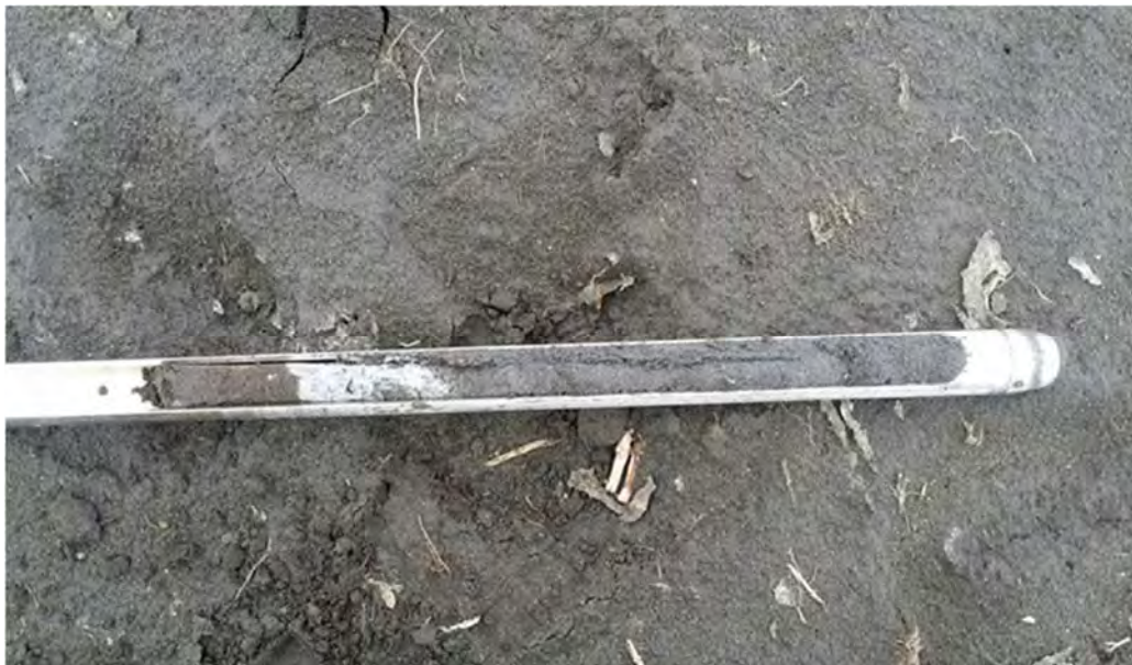
Photo 1 An example of an extracted soil core
