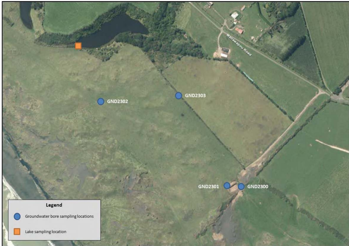
Figure 4 Groundwater monitoring bore sampling sites at the Symes Manawapou Landfarm
