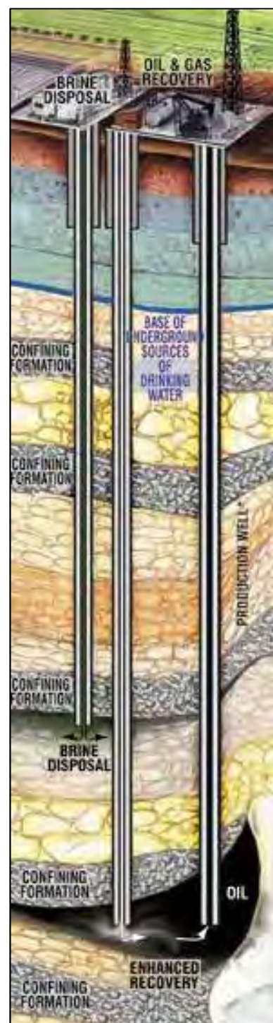
Figure 1 DWI schematic ( www.epa.gov/uic )
