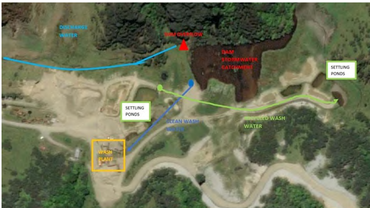
Photo 24 Uruti quarry, site map of lower wash water, excluding new laydown area for stockpiling, July 2021
