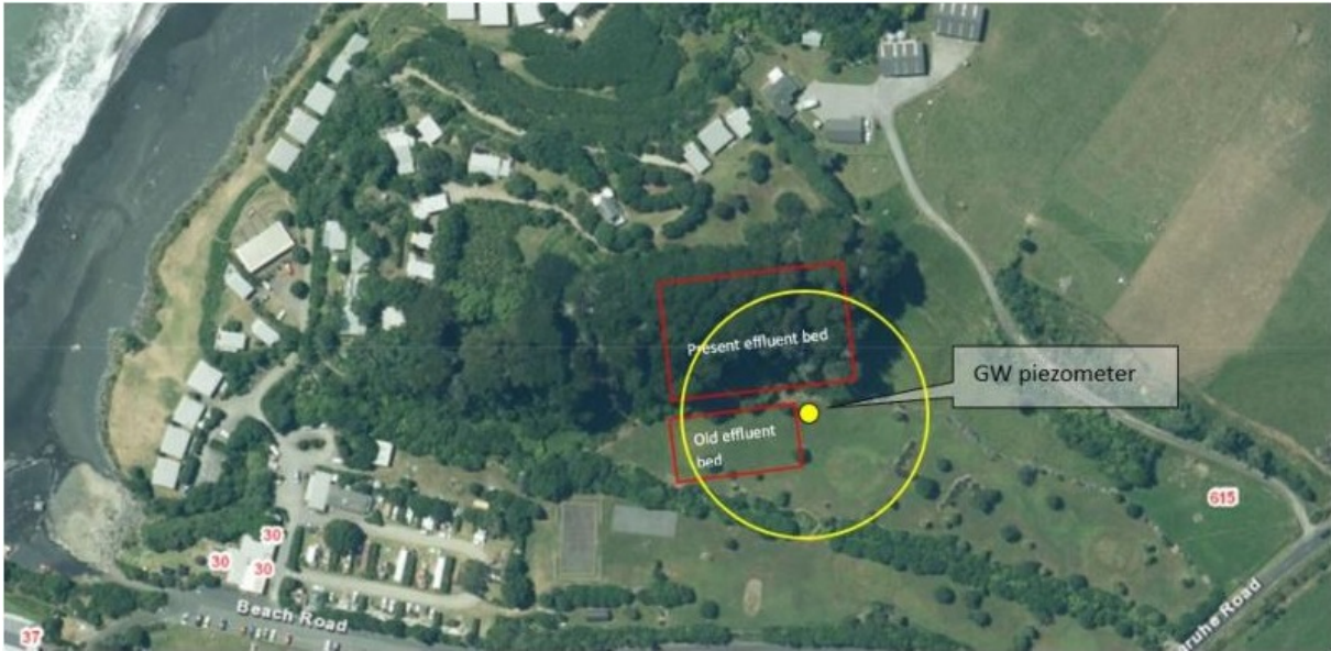
Figure 2 Location of the new piezometer/GND3189 in relation to the old and present effluent beds. The yellow circle represents a 50m radius
