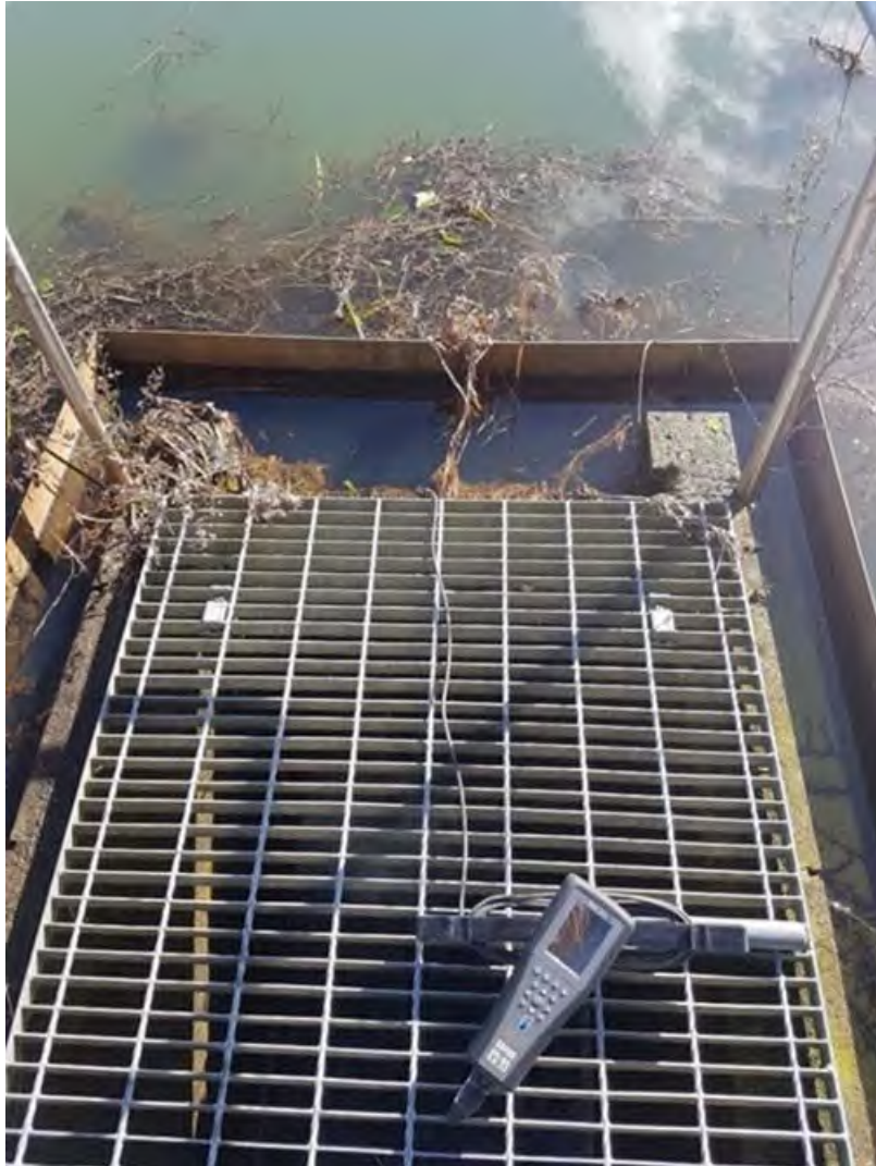
Photo 3 Dissolved oxygen monitoring
