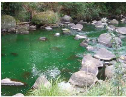
Photo 2 Dye tracing in the Patea River at the boundary of the mixing zone, March 2014
