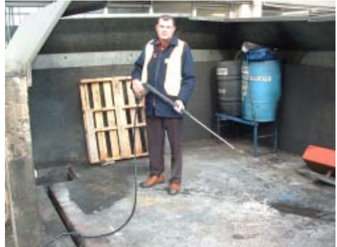
Photo 1: Wastewater from water blasting should be contained for appropriate disposal
