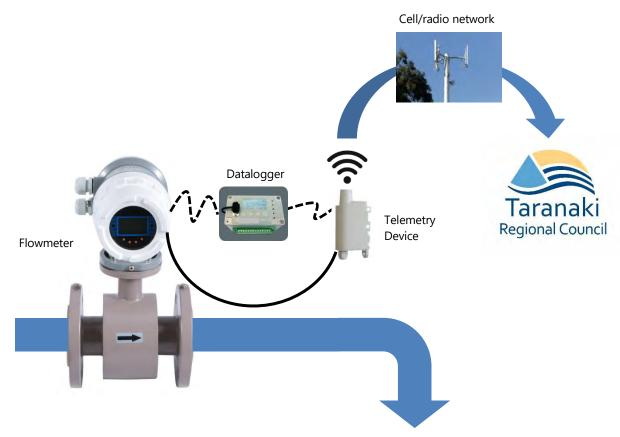
A typical set-up with a flowmeter (measuring device), a datalogger (water usage recording device) and a telemetry device. In some cases, a datalogger will not be required.
