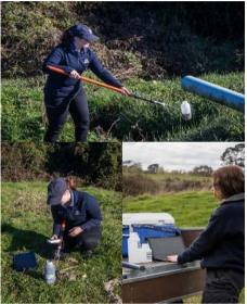
Photo 4 Collecting samples, recording temperature and entering sample information into the laboratory database remotely
